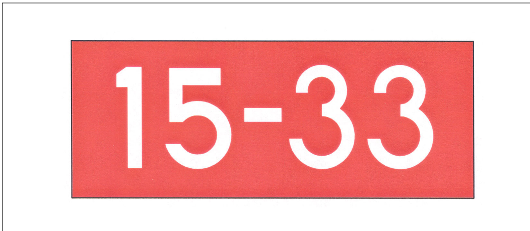
FIG 2-3-24 Runway Holding Position Sign
