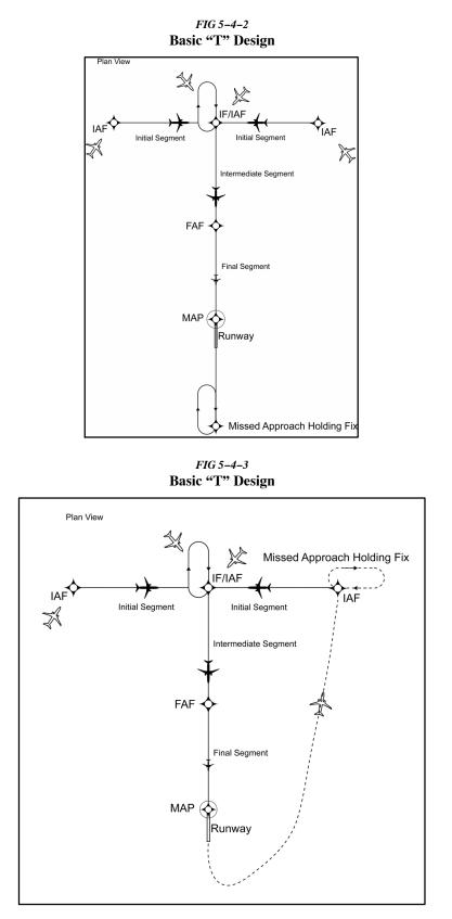
**3.** The standard TAA based on the "T" design consists of three areas defined by the Initial Approach Fix (IAF) legs and the intermediate segment course beginning at the IF/IAF. These areas are called the straight-in,
