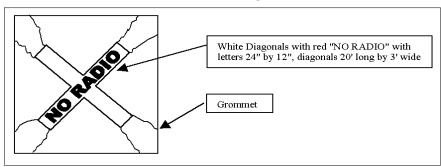
FIG 10-2-1 Closed Helideck Marking – No Radio
