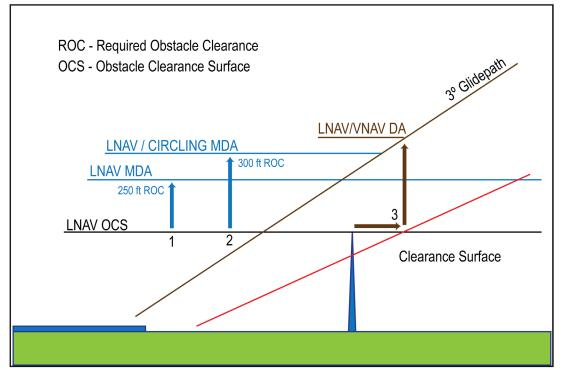
**g.** FIG 5–4–13 provides a visual representation of an obstacle evaluation and calculation of LNAV MDA, Circling MDA, LNAV/VNAV DA.
