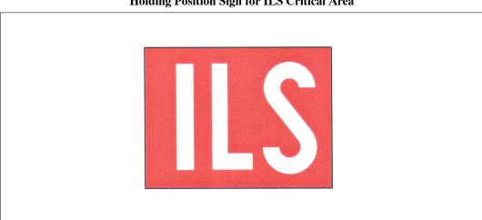
FIG 2-3-28 Holding Position Sign for ILS Critical Area
