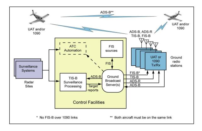
*FIG* 4–5–6 ADS–B, TIS–B, and FIS–B: Broadcast Services Architecture
