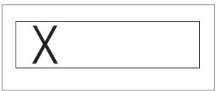
**d.** Marking and Lighting of Permanently Closed Runways and Taxiways. For runways and taxiways which are permanently closed, the lighting circuits will be disconnected. The runway threshold, runway designation, and touchdown markings are obliterated and yellow crosses are placed at each end of the runway and at 1,000 foot intervals. (See FIG 2–3–22.)
