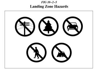
**5.** Keep spectators back at least 200 feet. Keep emergency vehicles 100 feet away and have fire equipment (if available) standing by. Ground personnel should wear eye protection, if available, during landing and takeoff operations. To avoid loose objects being blown around in the LZ, hats should be removed; if helmets are worn, chin straps must be securely fastened.
