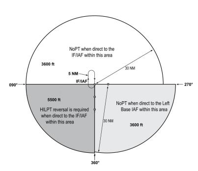
FIG 5-4-9 TAA with Right Base Eliminated
