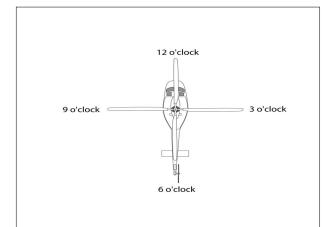
FIG 10-2-6 "Clock" System for Identifying Positions Relative to the Nose of the Aircraft
