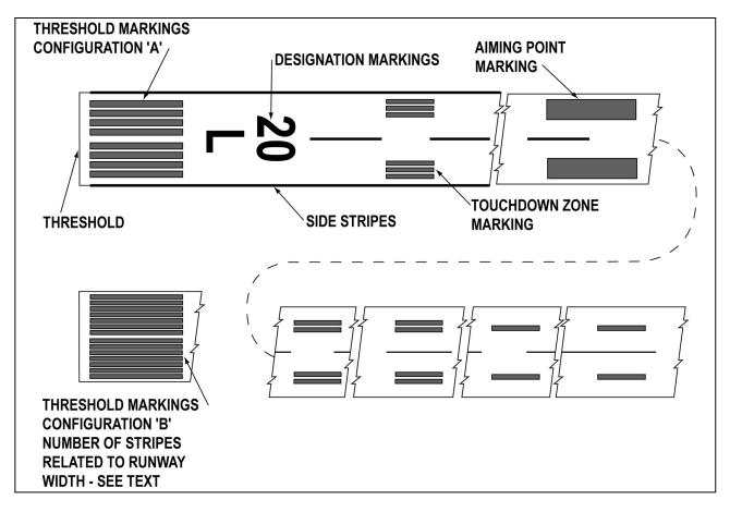
**b.** Runway Designators. Runway numbers and letters are determined from the approach direction. The runway number is the whole number nearest one-tenth the magnetic azimuth of the centerline of the runway, measured clockwise from the magnetic north. The letters, differentiate between left (L), right (R), or center (C) parallel runways, as applicable:
