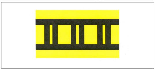
**4. ILS Critical Area Boundary Sign.** This sign has a yellow background with a black inscription with a graphic depicting the ILS pavement holding position marking as shown in FIG 2–3–34. This sign is located adjacent to the ILS holding position marking on the pavement and can be seen by pilots leaving the critical area. The sign is intended to provide pilots with another visual cue which they can use as a guide in deciding when they are "clear of the ILS critical area."
