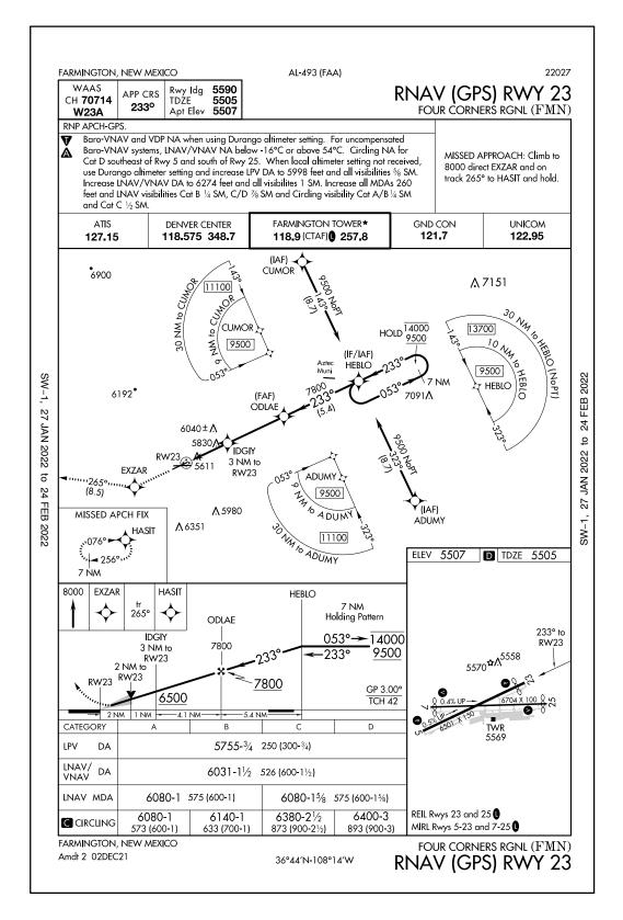
7. TAAs may be modified from the standard size and shape to accommodate operational or ATC requirements. Some areas may be eliminated, while the other areas are expanded. The "T" design may be modified by the procedure designers where required by terrain or ATC considerations. For instance, the "T" design may appear more like a regularly or irregularly shaped "Y," upside down "L," or an "I."
