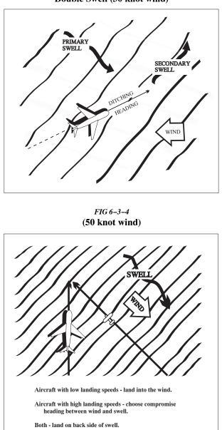
FIG 6-3-5 Wind-Swell-Ditch Heading
