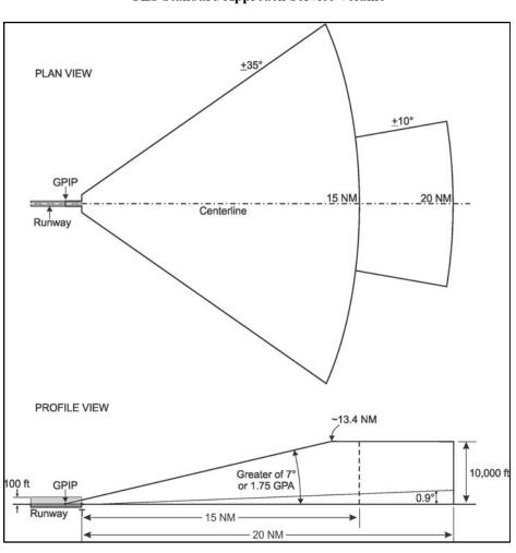
*FIG 1–1–9* GLS Standard Approach Service Volume
