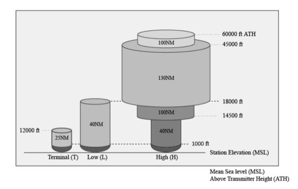
*FIG 1–1–2* Lower Edge of the Terminal Service Volume (in altitude ATH)
