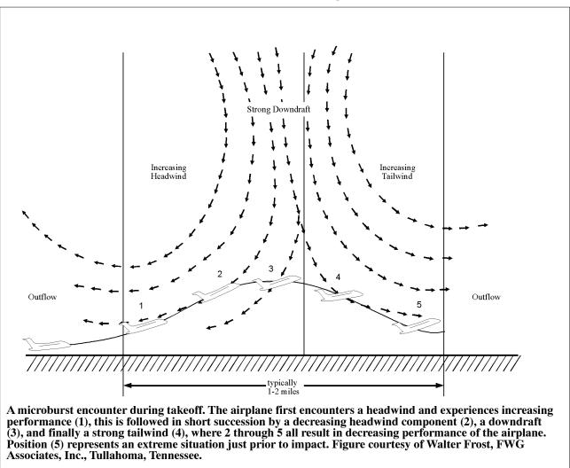
e. Microburst wind shear may create a severe hazard for aircraft within 1,000 feet of the ground, particularly during the approach to landing and landing and take-off phases. The impact of a microburst on aircraft which have the unfortunate experience of penetrating one is characterized in FIG 7–1–14. The aircraft may encounter a headwind (performance increasing) followed by a downdraft and tailwind (both performance decreasing), possibly resulting in terrain impact.
