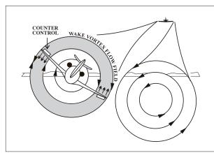
FIG 7-4-2 Wake Encounter Counter Control
