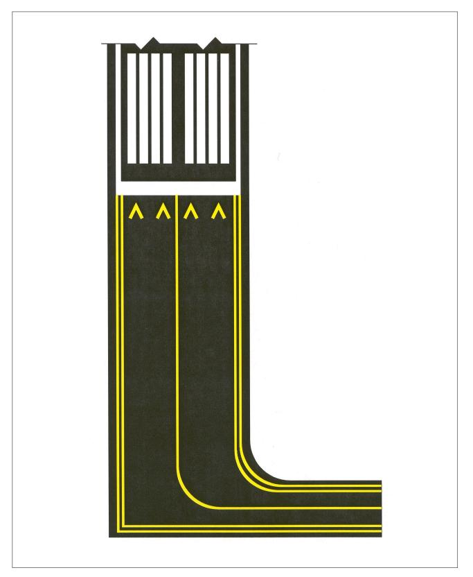
FIG 2-3-4 Displaced Threshold Markings
