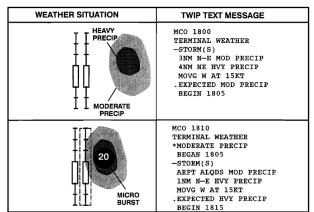
*FIG 7–1–21* TWIP Image of Convective Weather at MCO International
