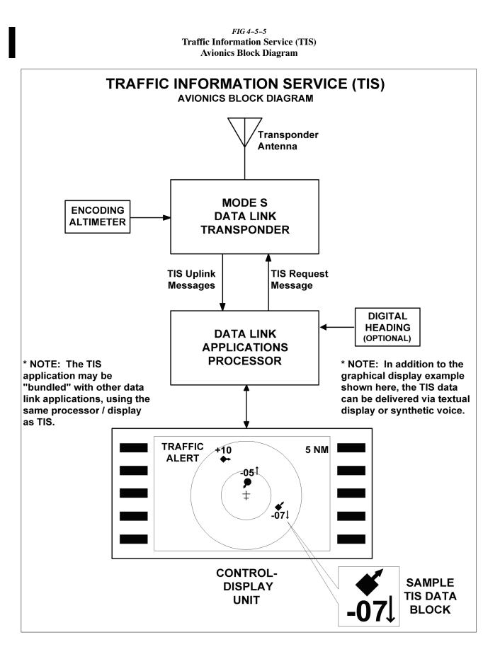
**2.** The cockpit equipment functionality required by a TIS client aircraft to receive the service consists of the following (refer to FIG 4-5-5):
