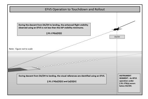
FIG 5-4-32 EFVS Operation to Touchdown and Rollout
