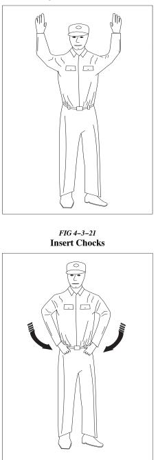
*FIG 4–3–22* Cut Engines
