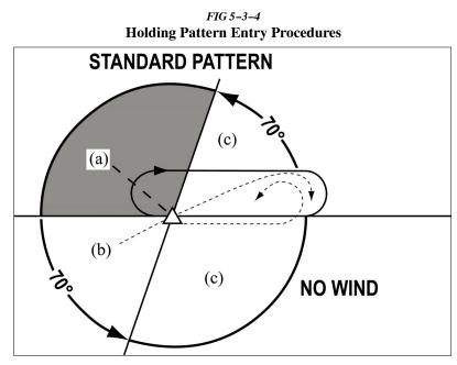
**3.** Entry Procedures. Holding protected airspace is designed based in part on pilot compliance with the three recommended holding pattern entry procedures discussed below. Deviations from these recommendations, coupled with excessive airspeed crossing the holding fix, may in some cases result in the aircraft exceeding holding protected airspace. (See FIG 5–3–4.)
