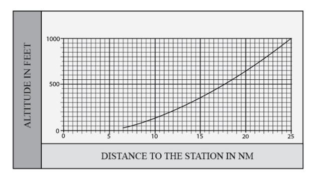
*FIG 1-1-3* Lower Edge of Low and High Service Volumes (in altitude ATH)
