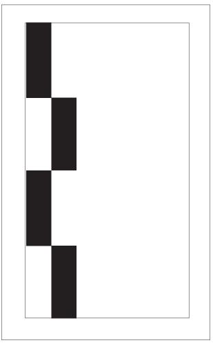
**c.** Nonmovement Area Boundary Markings. These markings delineate the movement area (i.e., area under ATC). These markings are yellow and located on the boundary between the movement and nonmovement area. The nonmovement area boundary markings consist of two yellow lines (one solid and one dashed) 6 inches (15cm) in width. The solid line is located on the nonmovement area side, while the dashed yellow line is located on the movement area is shown in FIG 2-3-21.
