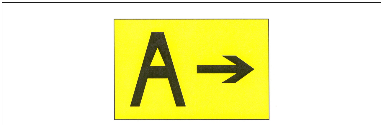
FIG 2-3-36 Direction Sign for Runway Exit
