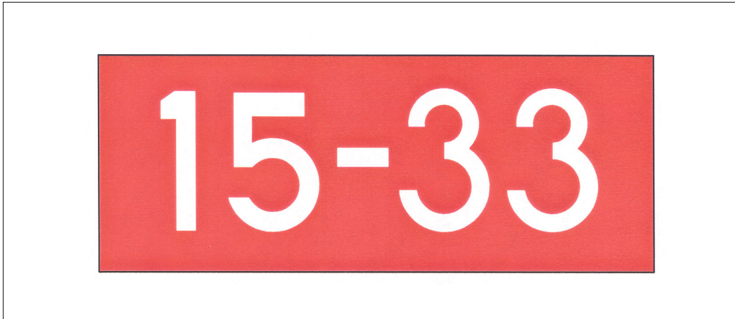
FIG 2-3-24 Runway Holding Position Sign
