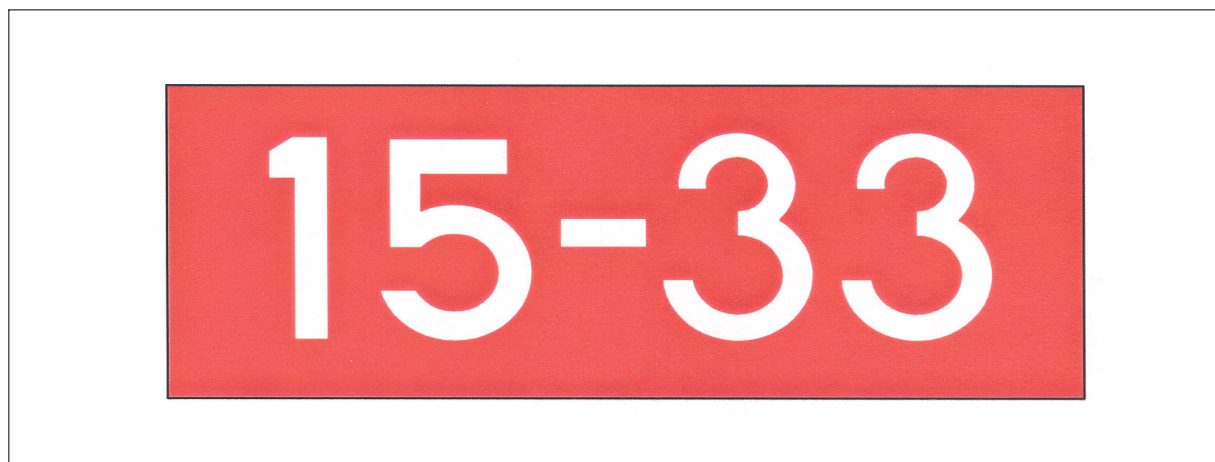
FIG AD 1.1-36 Runway Holding Position Sign
