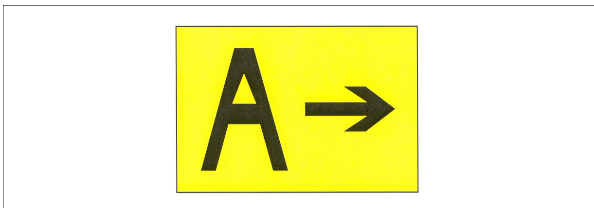
FIG AD 1.1-48 Direction Sign for Runway Exit
