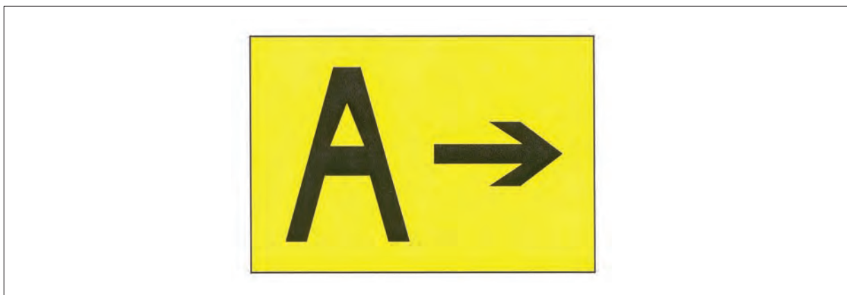
FIG AD 1.1-48 Direction Sign for Runway Exit
