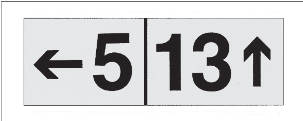
FIG AD 1.1-52 Destination Sign for Different Taxiing Routes to Two Runways
