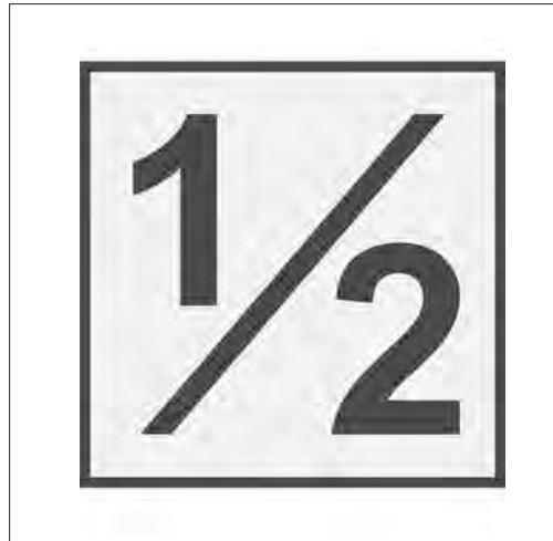
FIG ENR 5.7-1 Typical Runway Half-way Sign
