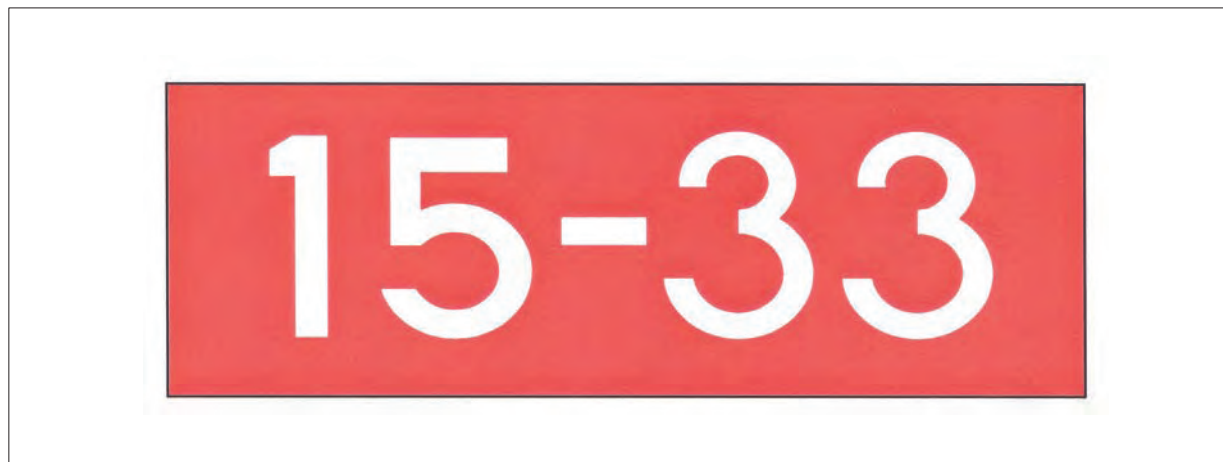
FIG AD 1.1-36 Runway Holding Position Sign
