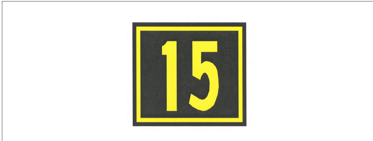
FIG AD 1.1-44 Runway Location Sign
