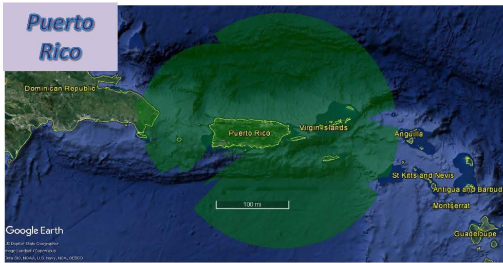
FIG ENR 1.6-4 Hawaii, Puerto Rico, and Guam with SSR Coverage at 5,000' AGL
