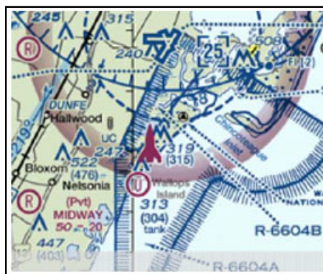
FIG ENR 5.7-3 Space Launch and Reentry Area Depicted on a Sectional Chart
