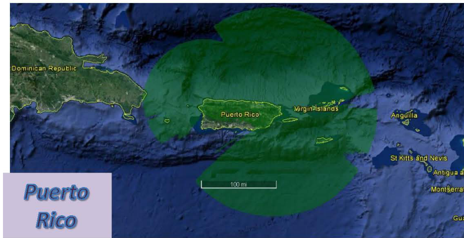
FIG ENR 1.6-3 Hawaii, Puerto Rico, and Guam with SSR Coverage at 1,500' AGL
