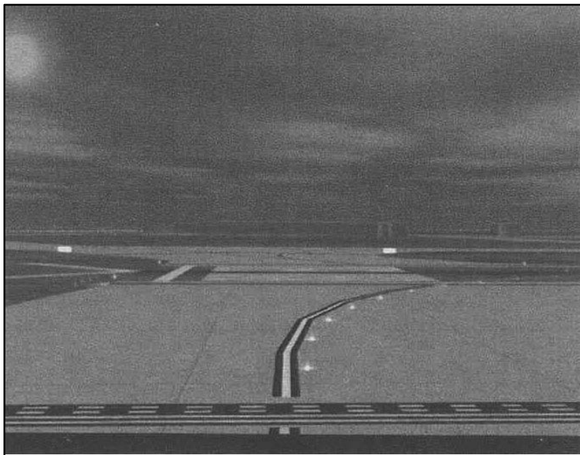
FIG AD 1.1-12 Taxiway Lead-On Light Configuration
