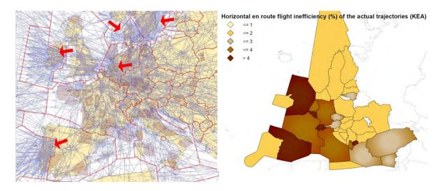
Figure 5.15: Flight efficiency improvements from free route implementation
