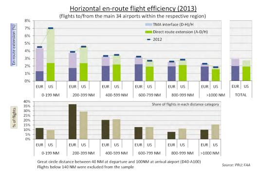
Figure 5.13: Comparison of total en route extension by component (2013)
