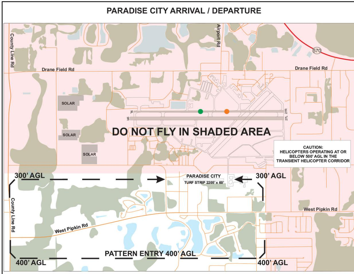
Paradise City turf strip is 2205 FT long x 60 FT wide with displaced thresholds on each end. A ditch runs parallel to the south side of the strip.
