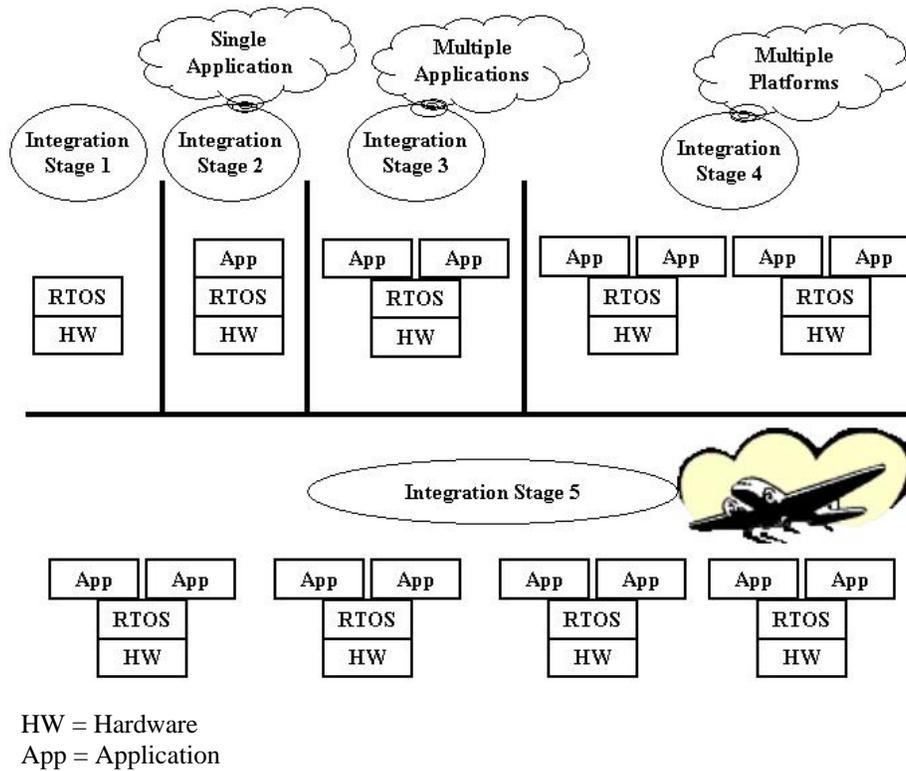
Figure 1. The IMA System Integration Stages
