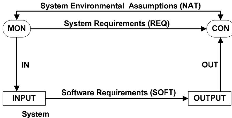
Figure 11. The Four-Variable Model
