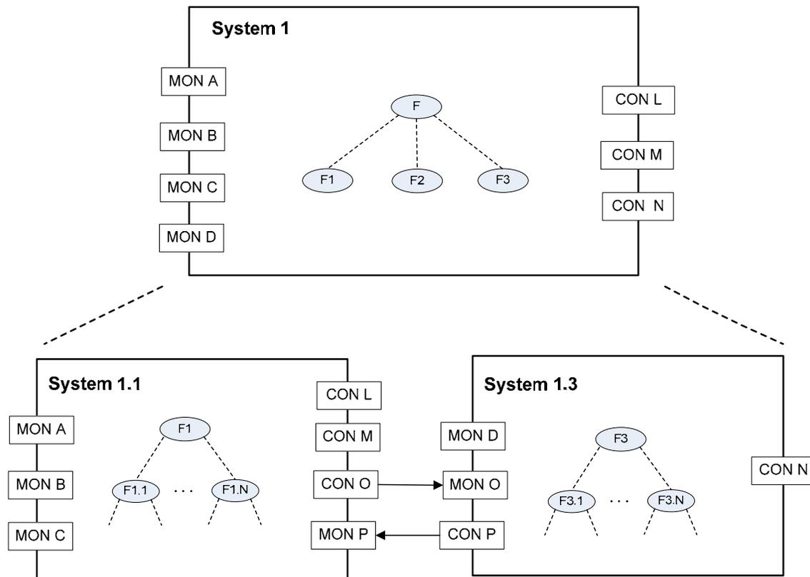
Figure 15. Decomposition of System 1 Into Subsystems
