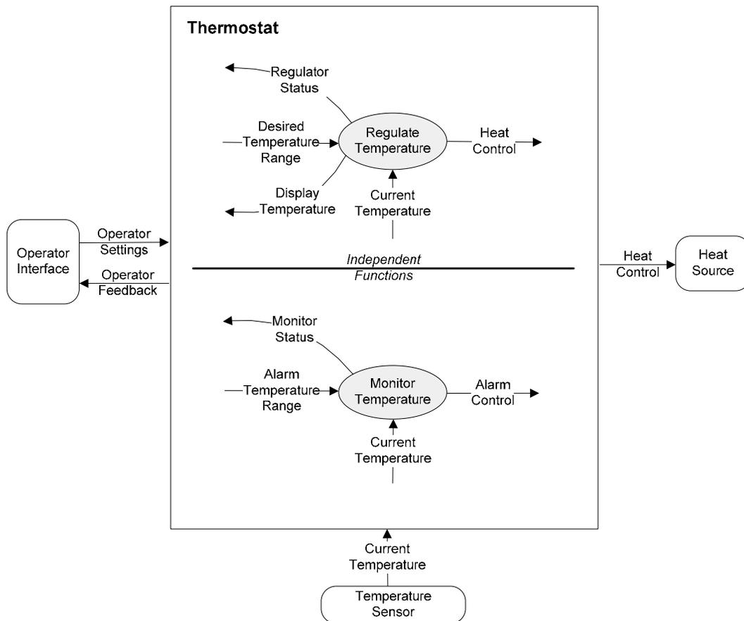
Figure 7. Revised Thermostat Dependency Diagram
