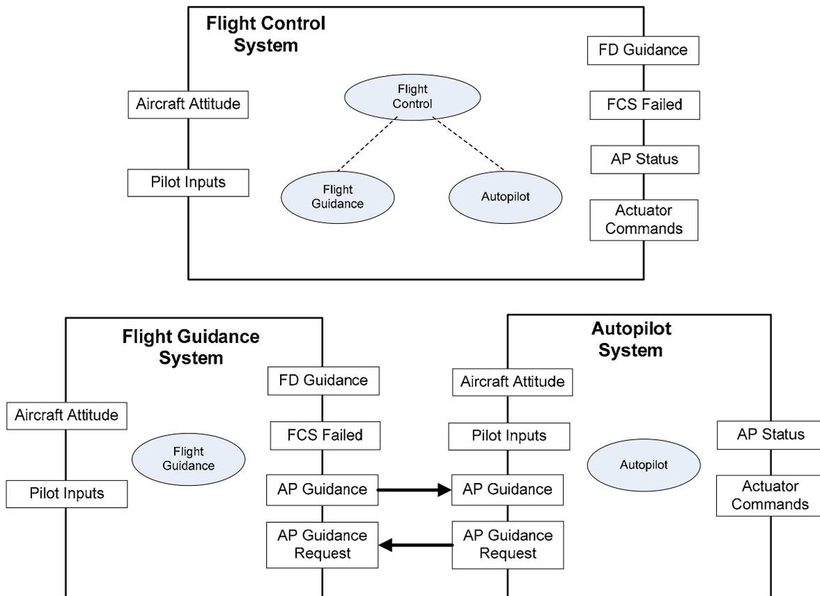
Figure 16. Allocation of FCS Requirements Into Subsystems
