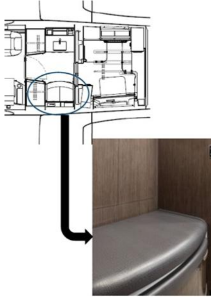
Figure 6: Toilet with Padded Seat Covering 1
