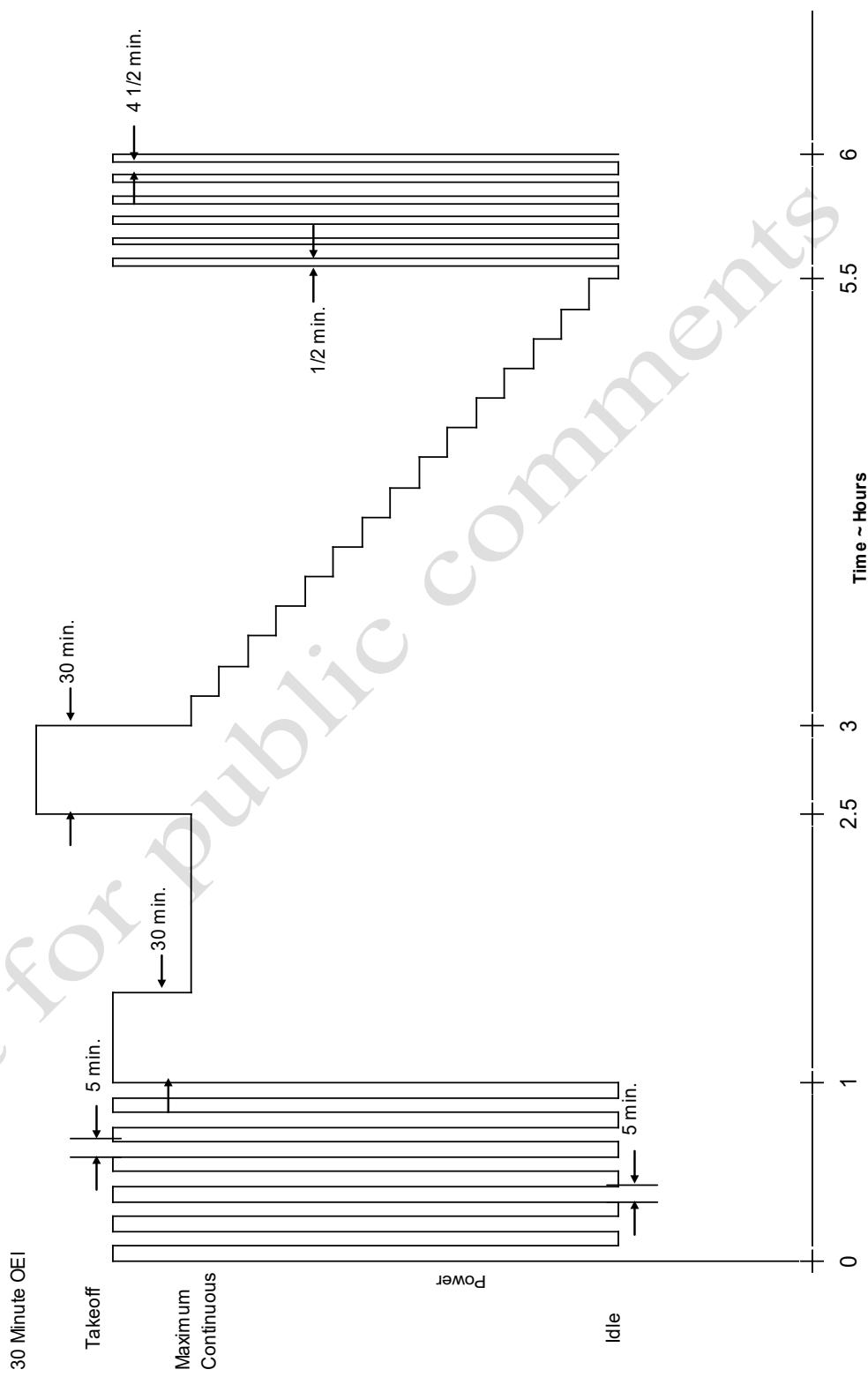
Figure 5. § 33.87(d), 150-Hour Endurance Test Cycles 1-15 for Rotorcraft Engine with Continuous OEI Power Rating
