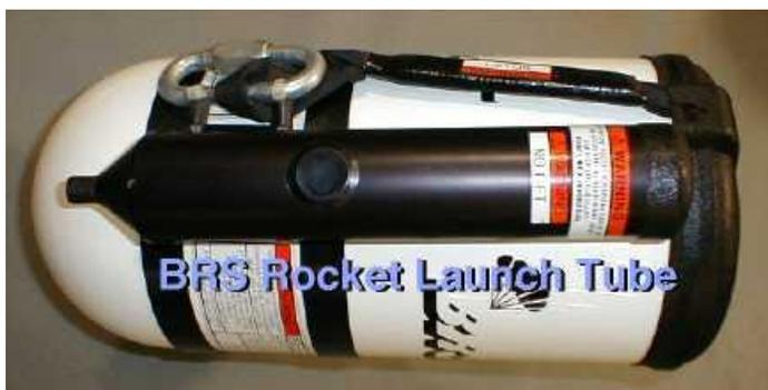
A rocket motor assembly consists of two principle parts: The launch body, which will leave the launch tube when fired; and the igniter, which remains in the launch tube after ignition. The launch tube on newer units is covered with a plastic cap while on certain older models it remained open.
