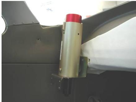
Here is another perspective of the **C172** rocket with cover removed. It is just a few inches below the rear window, which it will readily break through when fired.
