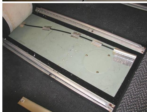
**Note:** This photo shows the routing of the activation cable between the front seats in either C172 or C182 installs. It is partially protected by aluminum channel, as you see in the right of the photo. Aluminum tape is also used to secure the cable to the floor. For any reason, should you be unable to access the cable near the igniter, this is a secondary point of access.
