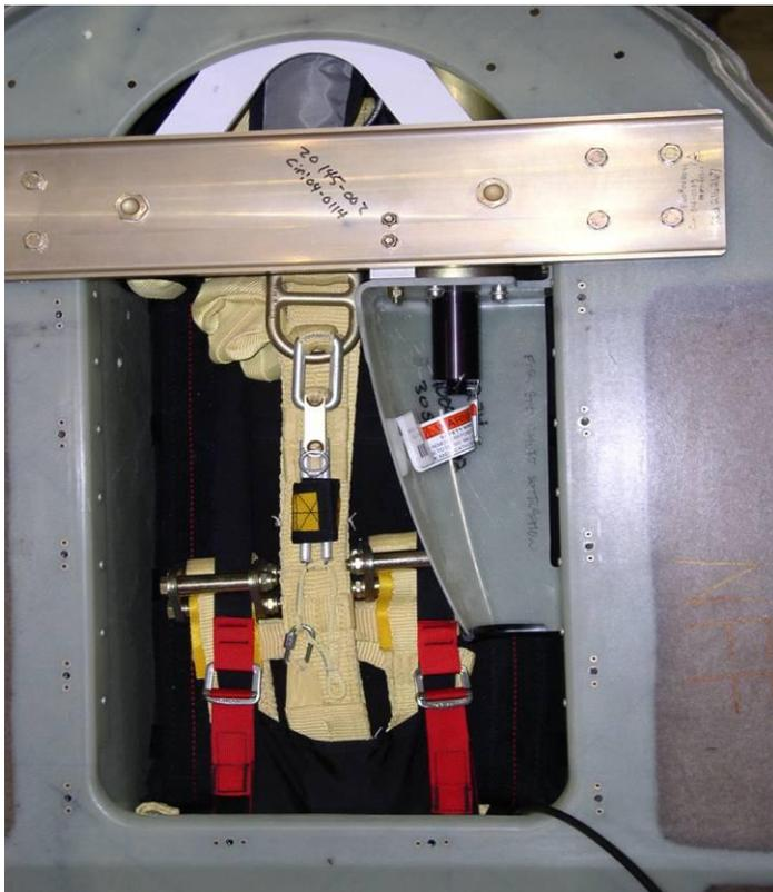
The photo at left shows the **Cirrus** parachute installed into its stowage area, located just behind the baggage compartment. It is normally covered by a sheet metal panel and interior trim. The rocket motor is mostly hidden behind the aluminum beam; the igniter is visible in the upper right center as a black cylinder. The Cirrus parachute is contained within a heavy nylon bag, so it is a *softpack* by definition.
