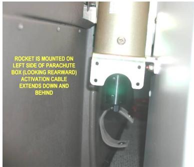
activation cable runs down to the floorboard, under a cover, then forward to the activation handle, located near the fuel selector.
