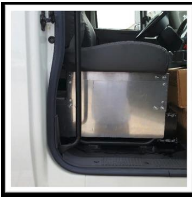
Installed aluminum safety enclosure
