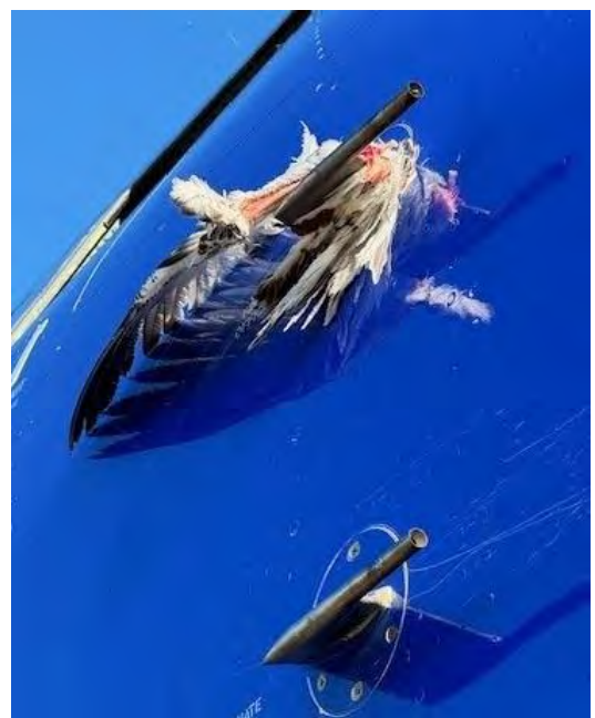
A B-737 800 struck a bird at 110 knots during take-off run at a west coast airport, February 2024. Pilot made a precautionary landing back at airport where bird remains were found in a pitot tube. Remains sent to Smithsonian were identified as white-headed gull complex. Photo, Airport.
