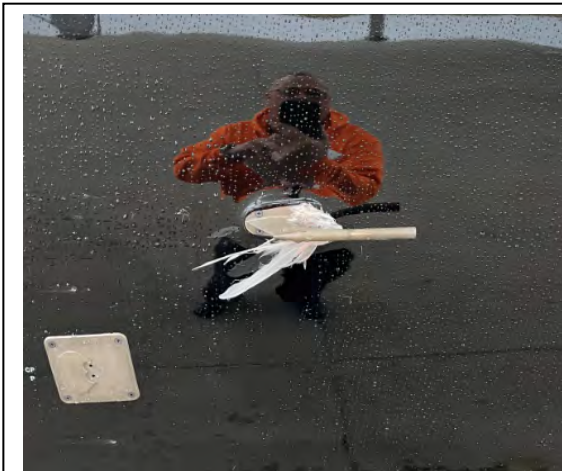
A Desault-2000 on approach to a midwestern airport in April 2024 struck a flock of ring-billed gulls at 20 feet AGL and 112 knots. The birds damaged the wing and struck the pitot tube (above). From 1990-2024, 928 pitot tubes have been reported as struck (48 in 2024). Ring-bills are the most frequently struck gull species for civil aircraft in USA. Photo, Airport.
