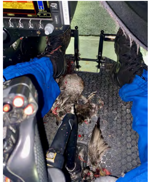
A ring-necked duck penetrated the chin bubble of a Eurocopter BK-117 on a medical mission in Massachusetts at midnight at 1,500 feet AGL and 110 knots, October 2024. The pilot, with duck remains at his feet, made an emergency landing at nearest airport. In 2024, there were 248 strikes with medical transport aircraft. Photo, Pilot.
