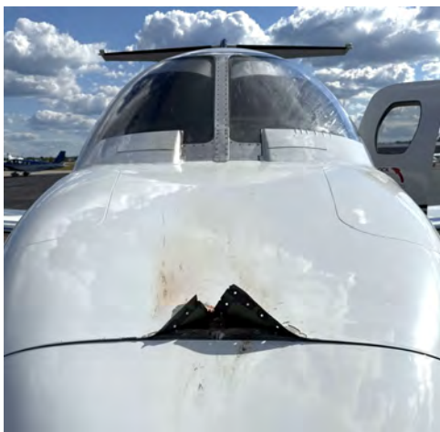
A Citationjet on approach to airport in Arkansas in Sept. 2024 struck a group of migrating broad-winged hawks at 5,800 feet AGL. Multiple birds were struck with damage to windshield, nose, and fuselage. Repair costs = $80,000; aircraft out of service = 60 hours. Photo, Pilot.
