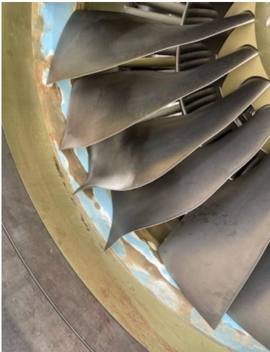
A B-737-800 ingested a “medium-sized” black bird (likely a vulture) in the #2 engine at 1200 feet AGL during climb out from an airport in Florida, September 2025. The pilot declared an emergency due to engine surges, reduced the engine to idle power, and made an emergency, overweight landing back at the airport. A record 138 strikes involving vultures (black and turkey) was reported in 2025. Photo, Airport.
