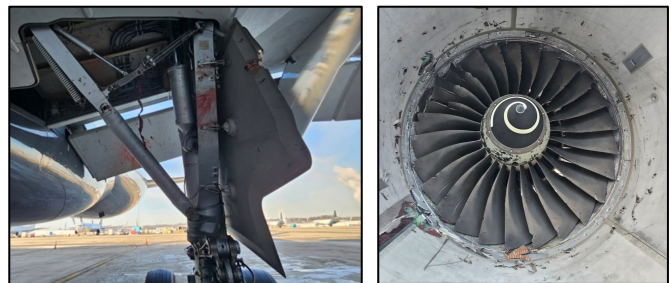
On January 28, 2026, an Airbus A330 (Amazon cargo flight operated by Alaska Airlines, Flight 2616) experienced a dual engine ingestion involving a minimum 8 Canada geese immediately following departure from CVG which resulted in significant engine and structural damage to the aircraft. Photos, Troy Levanen, Alaska Airlines.
