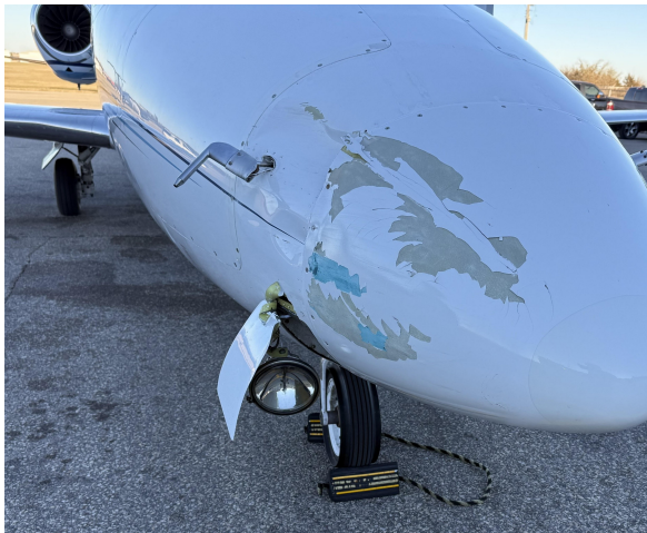
A BE-400 hit a bald eagle at 106 knots during take-off rotation from airport in Michigan, November 2025. The strike disabled the pitot tube and damaged the fuselage and landing gear door. From 1990-2025, 977 pitot tubes have been reported as struck (43 in 2025). Photo, Pilot.
