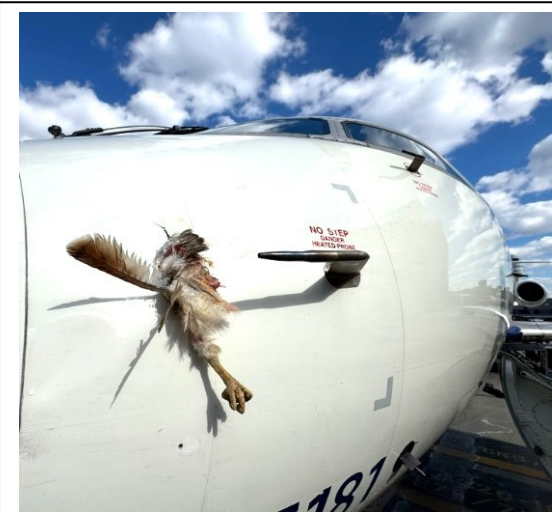
A CRJ900 on approach to an airport in Georgia in January 2025 struck a red-tailed hawk at 600 feet AGL. The bird penetrated the nose just forward of the pitot tube. The aircraft was taken out of service for repairs, Photo, Pilot.
