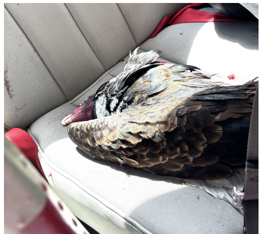
A Cessna 172 on approach to a Florida airport struck a turkey vulture at 1000 feet AGL and 100 knots, November 2025. The vulture hit the propeller and then shattered the windshield. The aircraft landed safely with no injuries to passengers or crew. Photo, Pilot.
