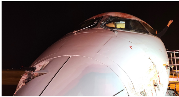
A CRJ100/200 on a 12-mile approach at night to an airport in Mississippi hit a flock of white-fronted geese at 3000 feet AGL, January 2025. The radome and nose had significant damage with minor damage to a winglet and vertical stabilizer. The impact caused the captain's primary flight display to become unusable, and the windshield was partially obscured by blood. Mitigation of strikes involving large migratory birds in these off-airport situations during climb and approach will require integration of avian radar and bird migration forecasting into airspace management for civil aviation. Photo, Airline.
