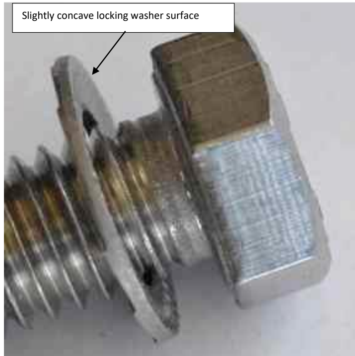
Figure 4. Bolt with a Slightly Concave Upper Locking Washer
