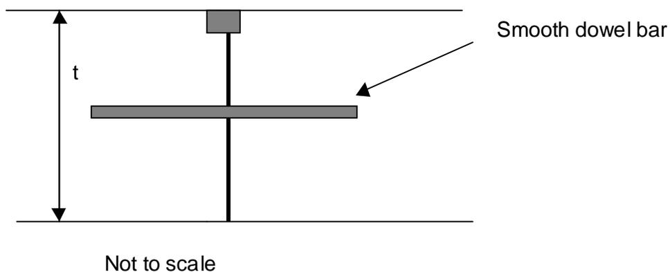
**Figure 14 - Doweled Construction Joint**
