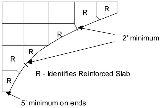
Figure 8 - Odd-Shaped Slab with Curved Edge
