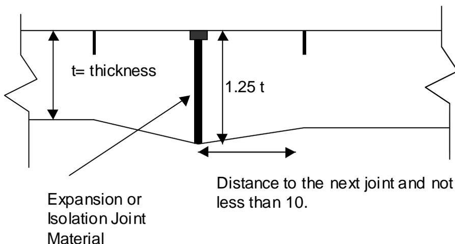
**Figure 12 - Thickened Edge Construction (Expansion / Isolation) Joint**
