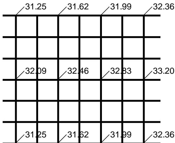
**Figure 7 - Grade Elevations at Joint Intersections**
