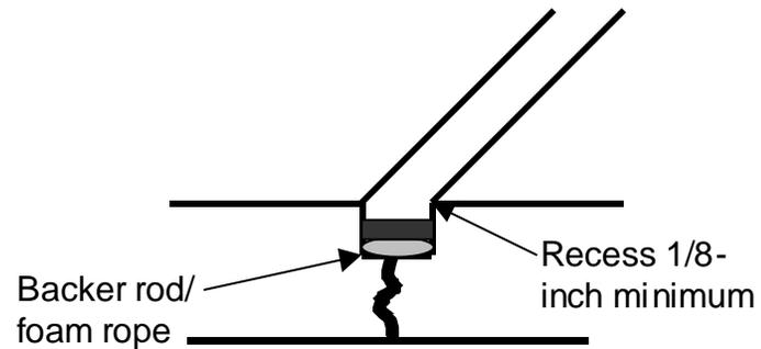
Figure 22 - Crack Repair
