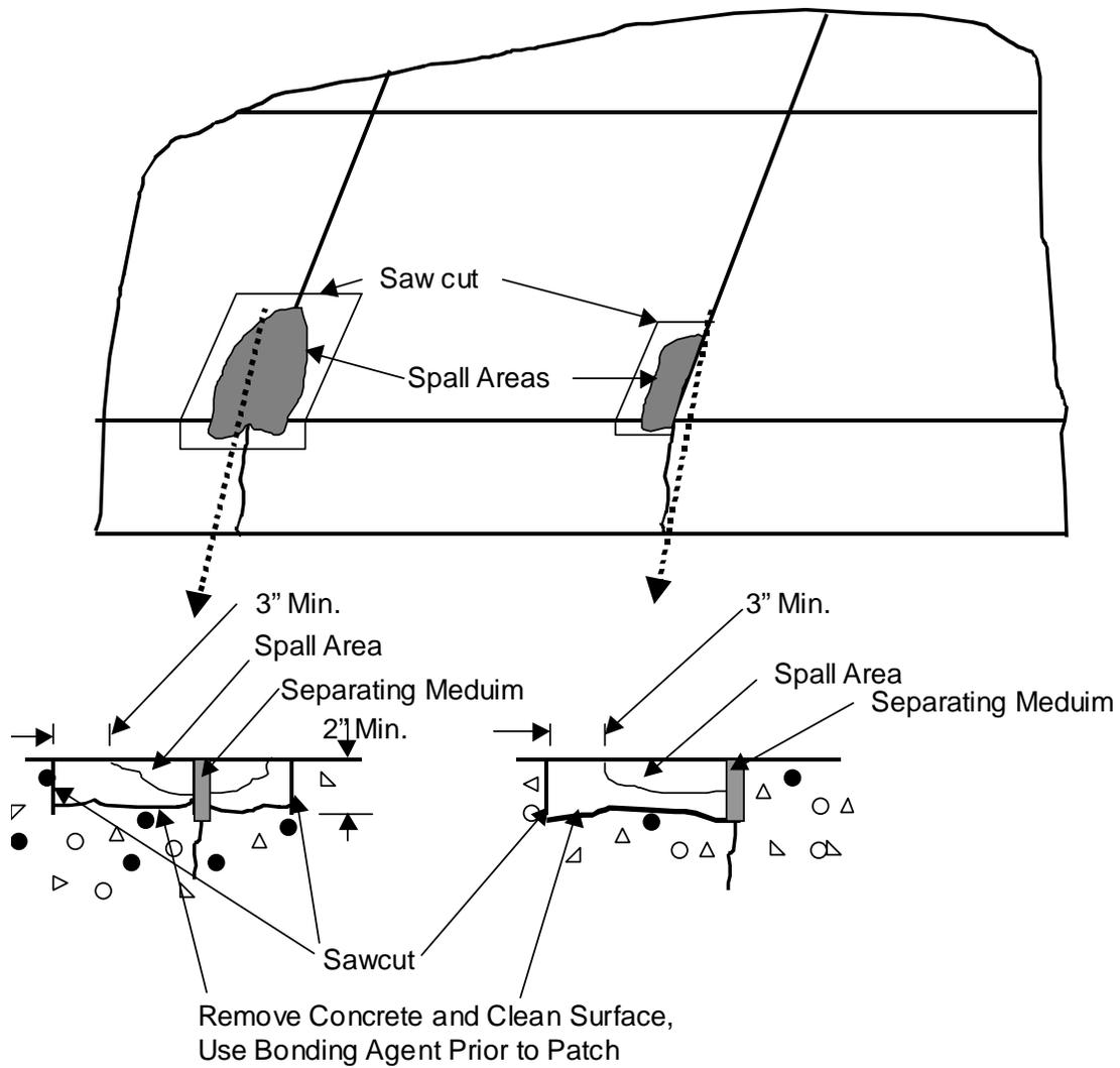
**Figure 23 - Spall Repair**
