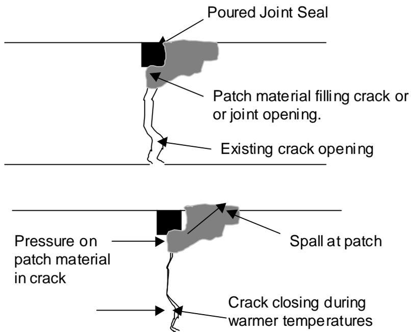
**Figure 21 - Spall Patching**
