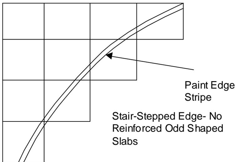
**Figure 10 - Odd-Shaped Slab with Stair-Stepped Edge**
