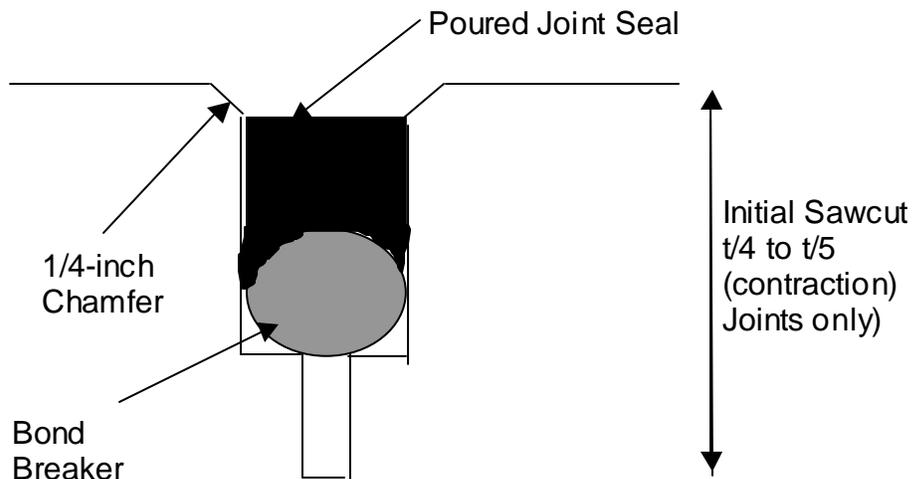
**Figure 20 - Joint Seal**
