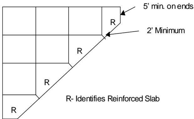
**Figure 9 - Odd-Shaped Slab with Straight Edge**
