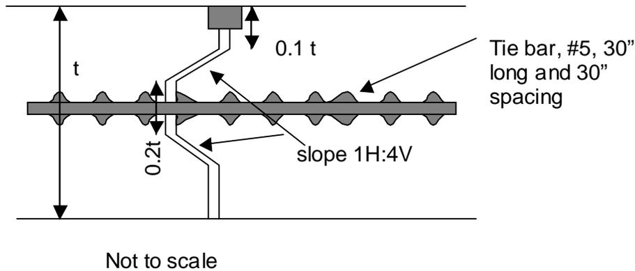
**Figure 13 - Keyed Construction Joint**
