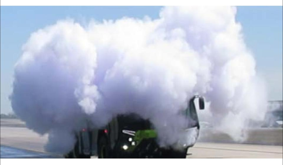
During the FAA inspection, vehicle operators may be requested to discharge a "quick puff" of dry chemical, during the timed response drill. Remember to check the wind!
