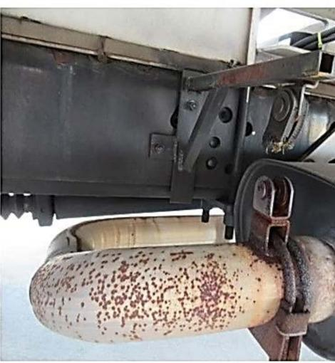
This fuel truck has a broken exhaust system hangar, which could lead to a future exhaust leak and potential fire safety issue.
