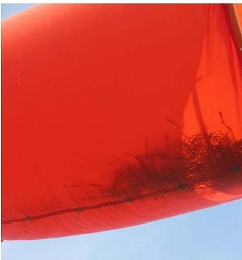
During daily inspections, wind cones must be inspected for visibility and operation. Water can also accumulate inside, if the drain holes are not installed properly.
