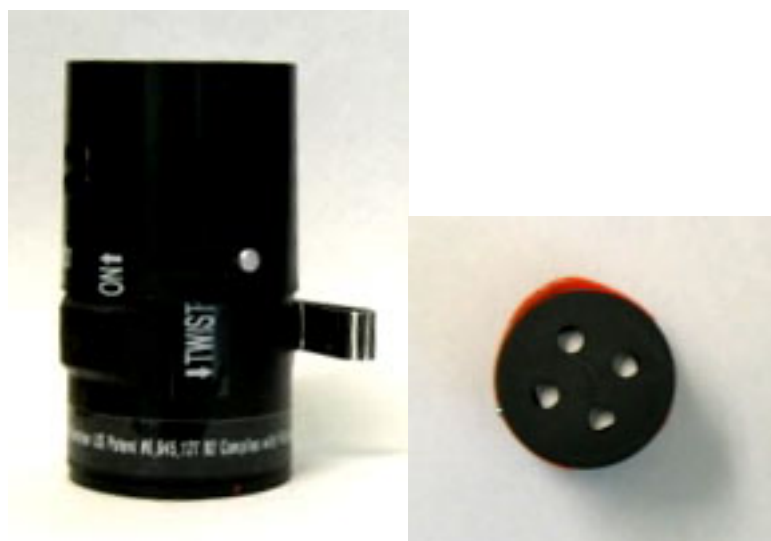
Figure 1: Side and top view of the van Netten sampler (on position), which is 9 cm in length, 5 cm in diameter.
