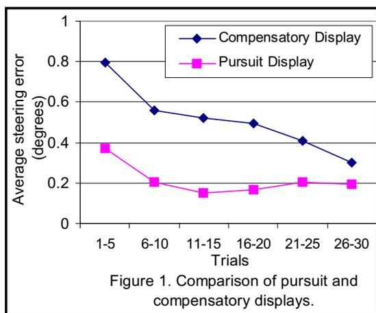
Figure 1. Comparison of pursuit and compensatory displays.
