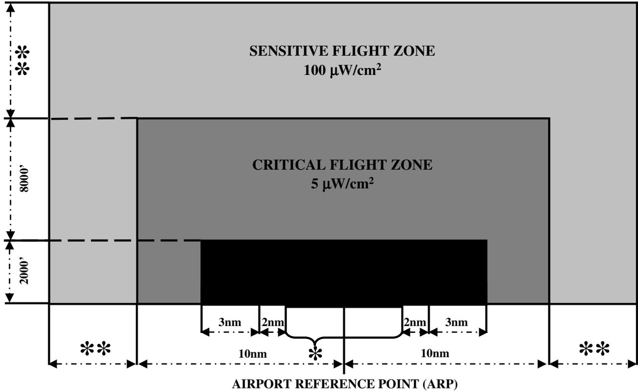
**Figure 1:** Profile view of a single-runway airport and the application of protected flight zones (Not drawn to scale). \* Runway length varies per airport. AGL is based on published airport elevation. \*\* To be determined by regional evaluation and/or local airport operations.
