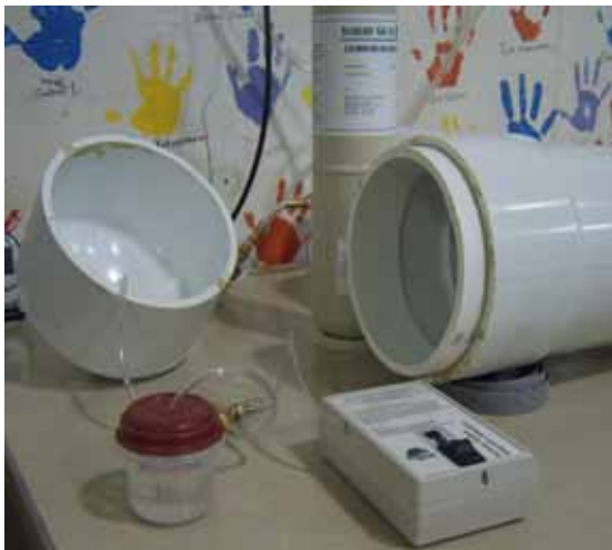
Figure 5. Altitude Chamber With CO 2 Calibration Gas
