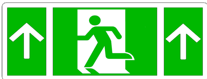
Figure 1: Approved Symbolic Exit Sign Featuring the ISO 7010:2011 Running Man With Narrow Arrows
