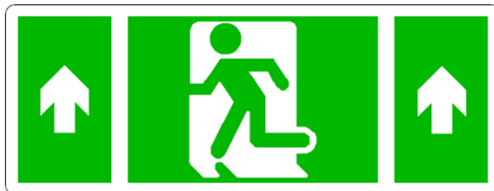
Figure 2: Proposed Symbolic Exit Sign Composed of a Modified ISO 7010:2011 Running Man and ISO 3864-3:2012 (E) Wide Arrows
