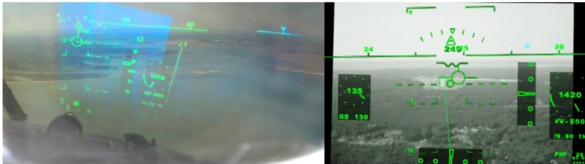
Figure 33 Pilot's View through HWD and HUD Symbolology.
