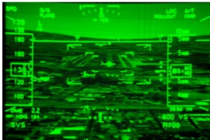
Fused HUD Concept with Tunnel
