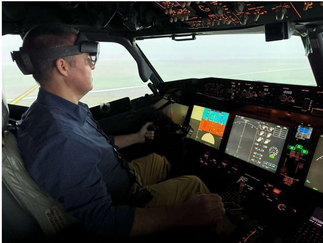
Figure 9 Microsoft HoloLens 2 in Simulator
