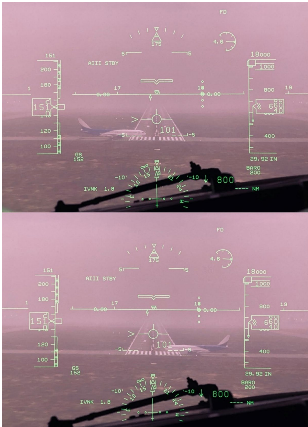
Images of Left and Right Runway Incursions Viewed Through the Head-Up Display
