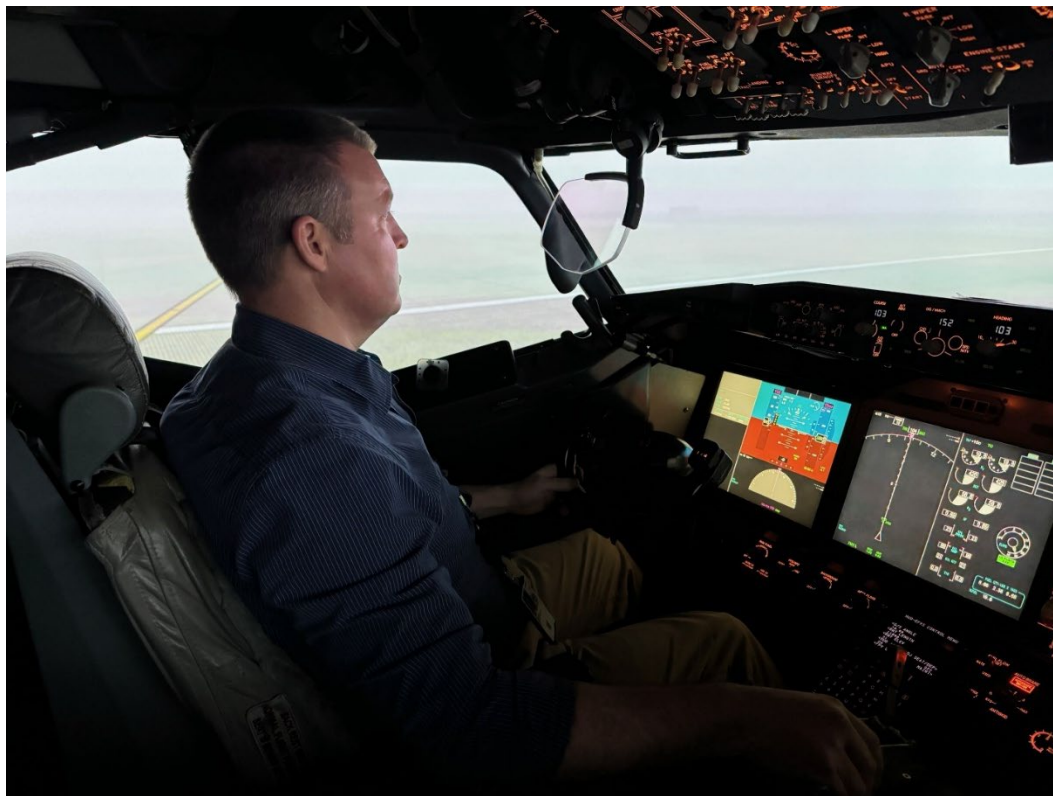
Collins Aerospace HGS-6700 Head-Up Display in Simulator
