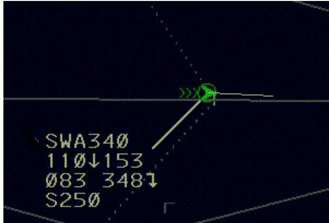
Figure 4. Chevron symbol denoting ADS-B equipage and aircraft directionality information.
