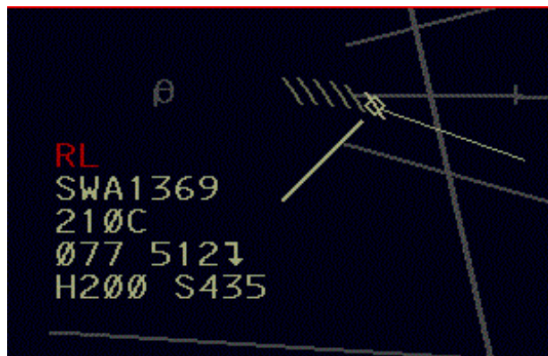
Figure 3. Red heading conformance violation alerts in line 0 of en route data blocks.
