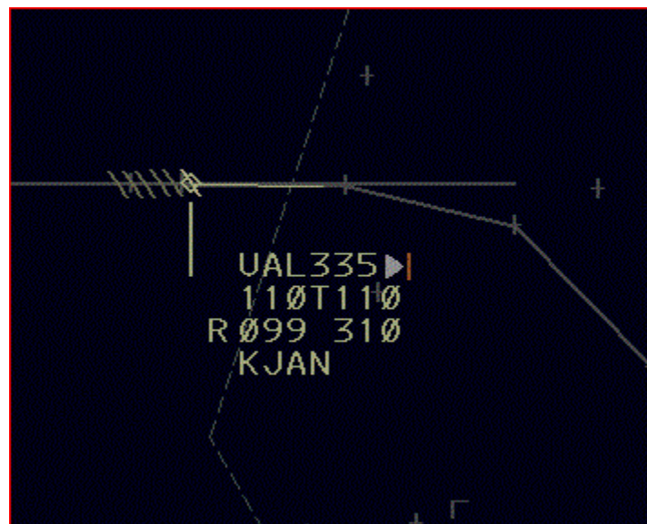
Figure 6. Symbol appended to data block indicating aircraft Data Comm capability.
