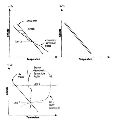
Figures 4-2a-c. Determination of atmospheric stability: (a) unstable case; (b) neutral case; (c) stable case.
