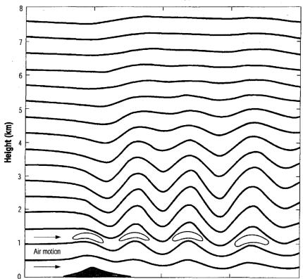
Figure 5-7. Lenticular clouds associated with a trapped lee wave (after Durran and Klemp).
