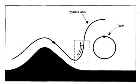
Figure 5-4. Schematic of the strong shear zone associated with a hydraulic jump in a mountain wave.
