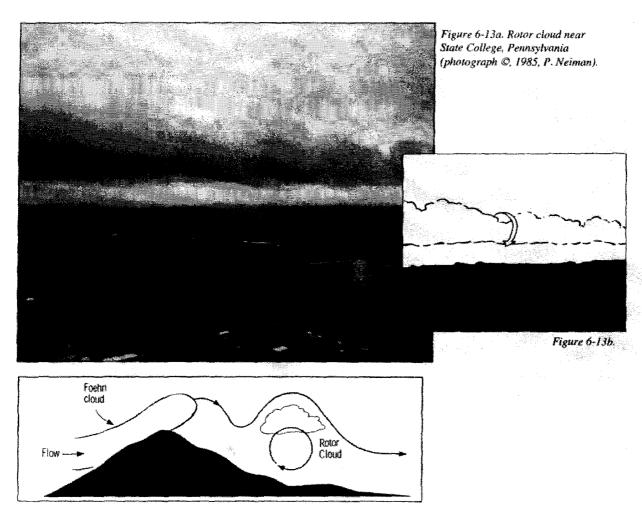
Figure 6-14. Schematic of the flow associated with a rotor zone in the lee of a mountain,
