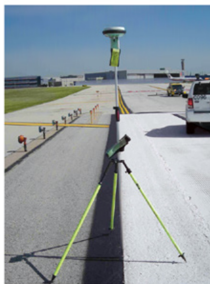
Correctly placed survey equipment
