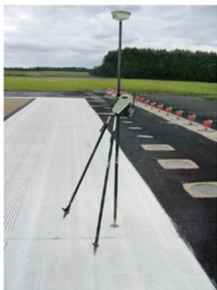
Incorrectly placed survey equipment
