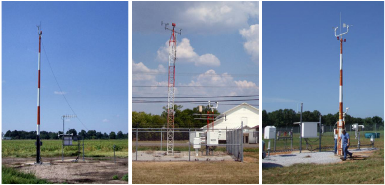
Figure 2-11. SAWS, AWOS and ASOS Station Installations.
