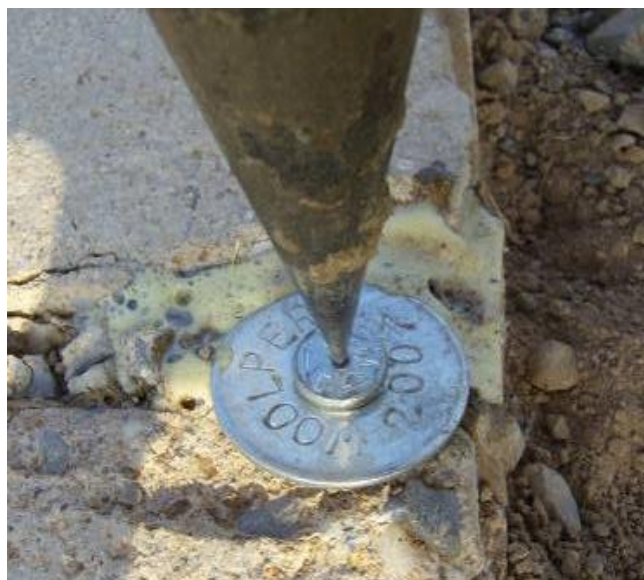
Figure 5-55. Close-up View of the Nail and Washer, Properly Inscribed.
