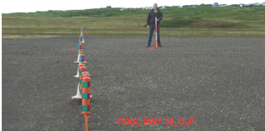
Figure 5-9. Shows the Location of the Runway Direction Point 10 Feet Inside the End Markers.
