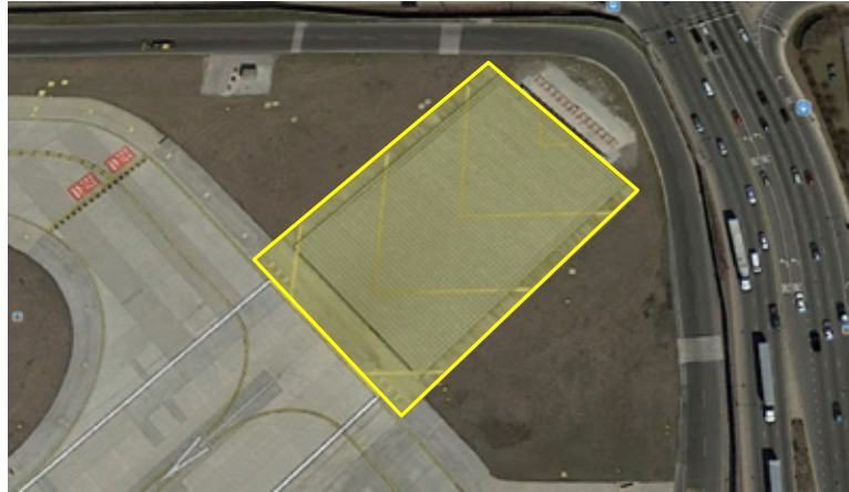
Figure 5-24. Runway 4L/22R EMAS at Chicago Midway Airport. Note the collection includes the setback value for the EMAS.
