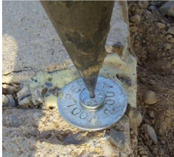
Figure 5-15. Provides a Close-up of the Nail and Washer Marking the Runway Direction Feature Location.
