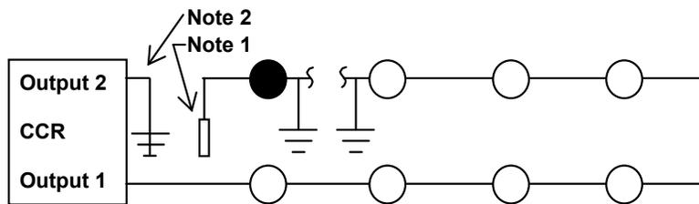
**Figure 6-10b. Grounded Output Test on CCR Output 2**
