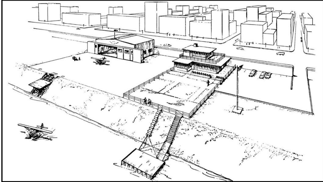
While some boat docks can be modified to accommodate seaplane access, the better solution is to specifically design a dock to accommodate seaplane access. When the seaplane base owner or sponsor is considering rehabilitation or reconstruction of an existing dock system the guidelines in this AC will prove helpful.
