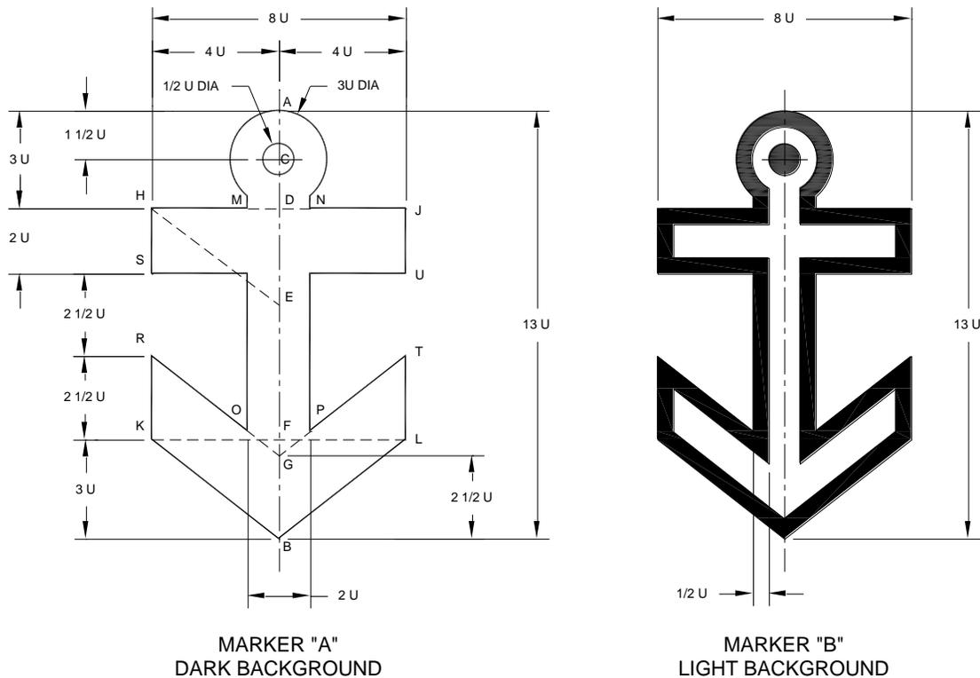
**Note:** Outside dimensions of markers are identical. Black border of marker "B" is 0.5 unit wide. One unit is 1/13 of the overall length.
