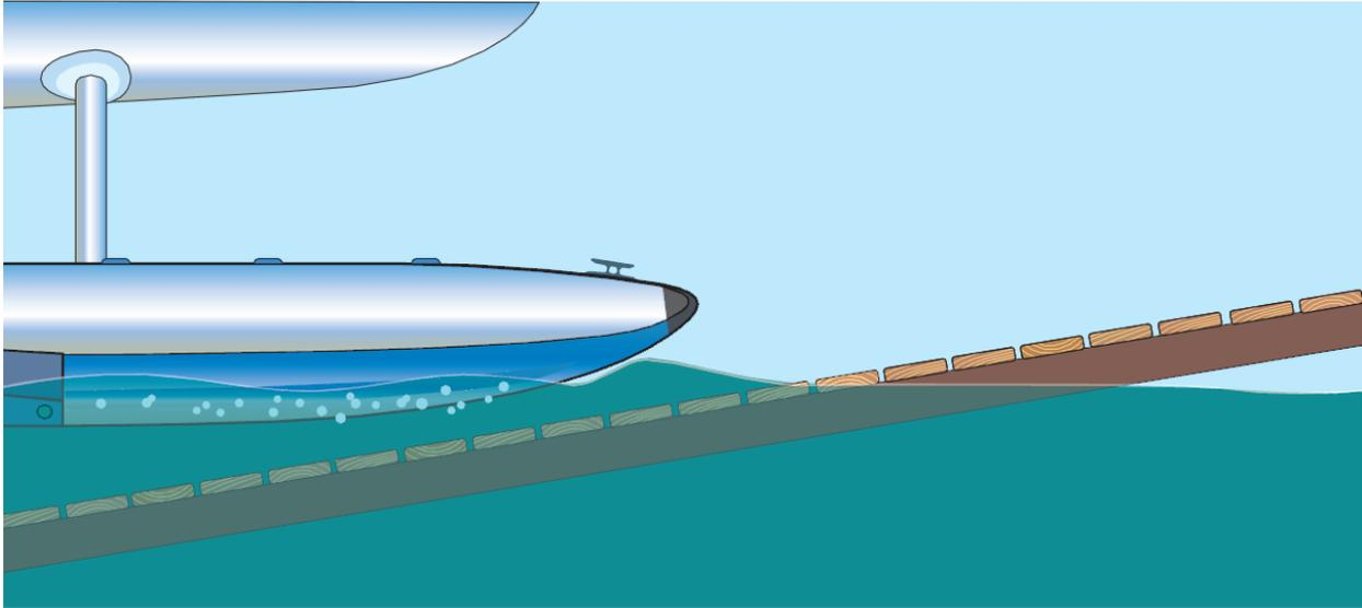
**Figure 4-3. Example of a Wood and Concrete Launch Ramp**
