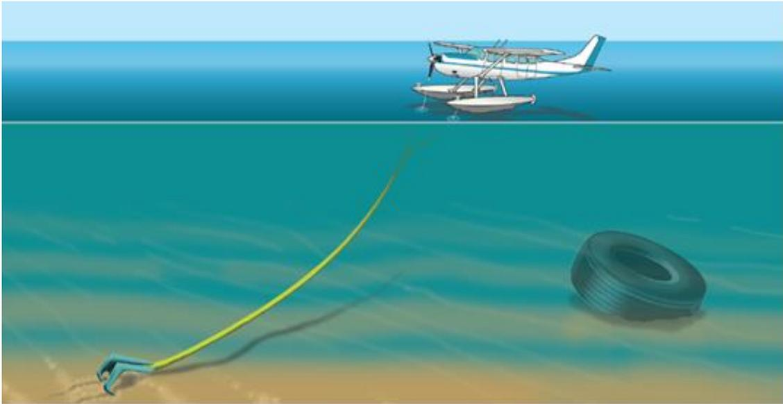
**Figure 3-7. Example of a Mooring Buoy Anchorage Area (Dual Anchor Line Plus Bridle)**
