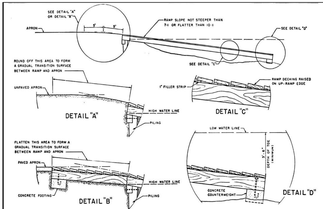
**Figure 4-2. Illustration of a Submerged Ramp Toe**
