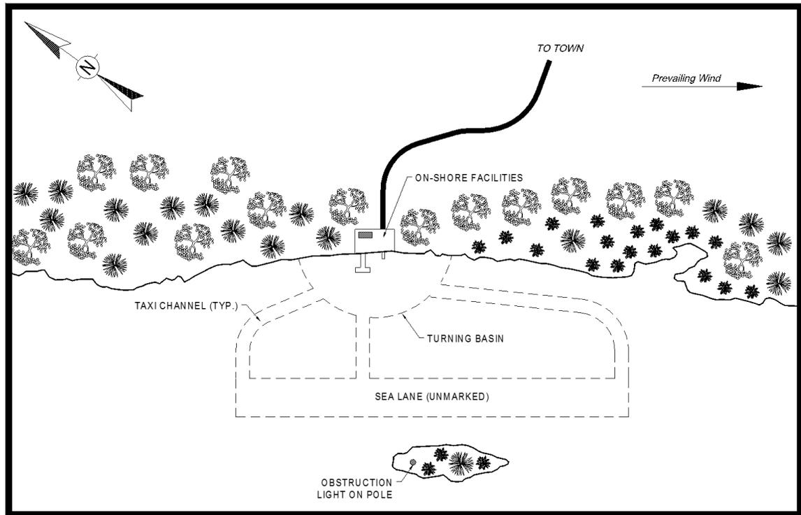
The disadvantage of unmarked water lanes is that aeronautical use surfaces, such as the approach and departure surfaces defined in AC 150/5300-13 and FAA Order 8260.3, United States Standard for Terminal Instrument Procedures (TERPS), as well as the 14 CFR Part 77 obstacle identification surfaces cannot be defined. This is because the surfaces are defined in relation to a marked runway threshold. An unmarked water lane does not have a defined threshold.
