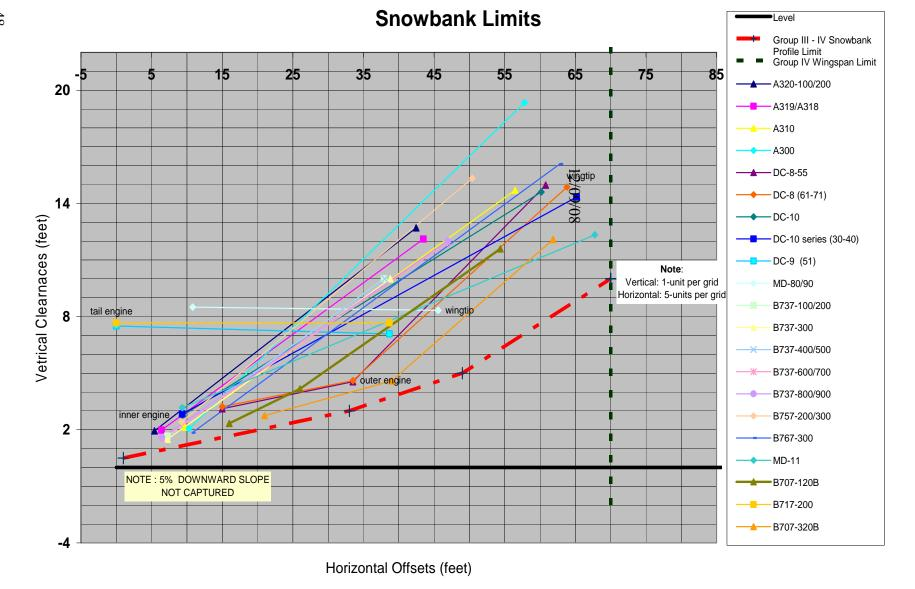
Graph A1-1. Individual height profiles of airplane wingtips and outer and inner engine nacelles' lower edges for Airplane Design Groups III and IV
