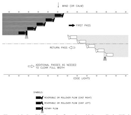
Figure 4-3. Possible Team Configuration with Perpendicular Wind (Dependent upon Rotary Plow performance)
