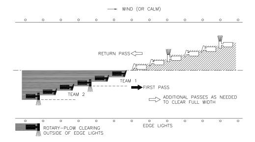
Figure 4-5. Possible Team Configuration During Medium to Heavy Snowfall with Parallel or Calm Wind (Dependent upon Rotary Plow performance)
