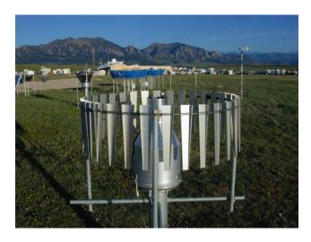
Figure 3-1. Single Alter Wind Shield Type
