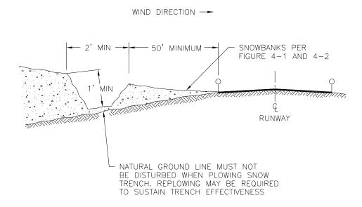
Figure 4-6. Typical Snow Trench Dimensions
