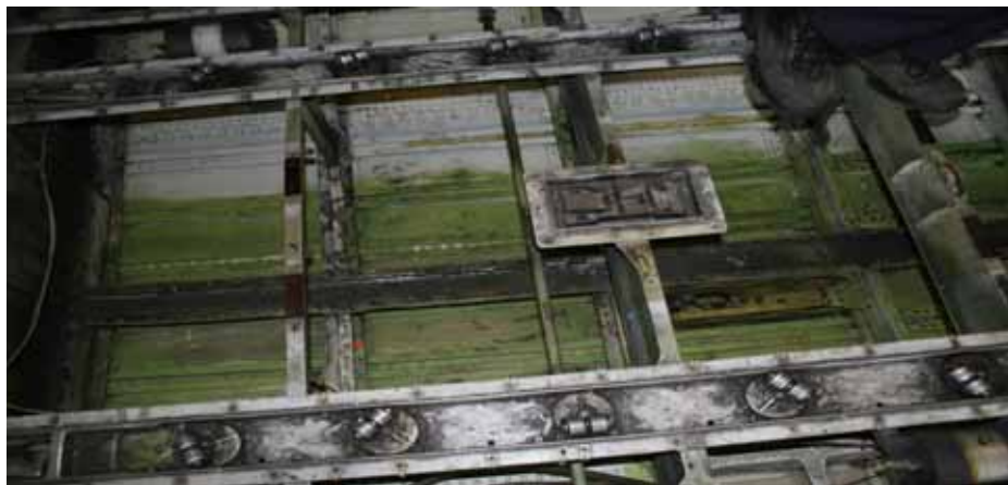
Figure 5-2. With the lower deck floor removed, the bilge bays can be more clearly seen. Water from firefighting will accumulate in the bilge.
