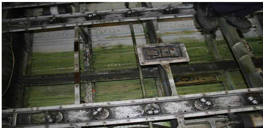
Figure 5-2. With the lower deck floor removed, the bilge bays can be more clearly seen. Water from firefighting will accumulate in the bilge.
