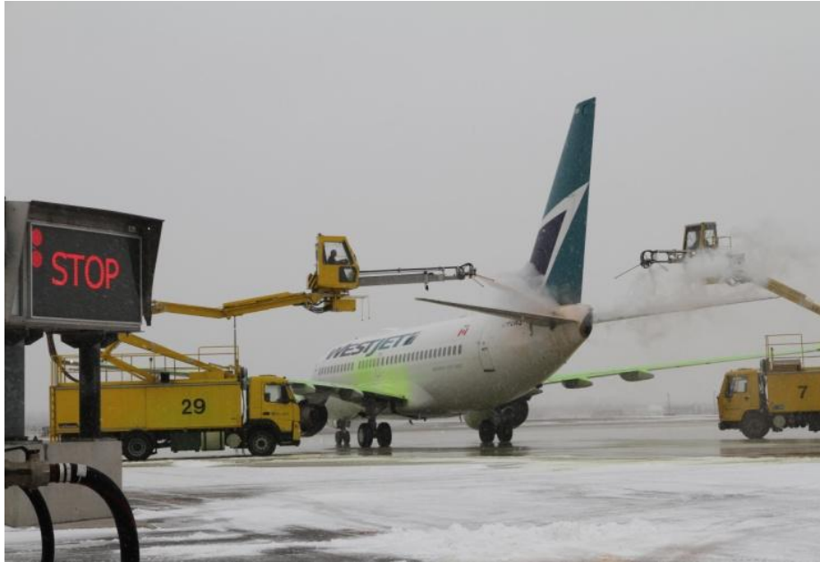
Figure 3-5(b). Electronic message board indicating the aircraft has reached the stop point of the deicing pad
