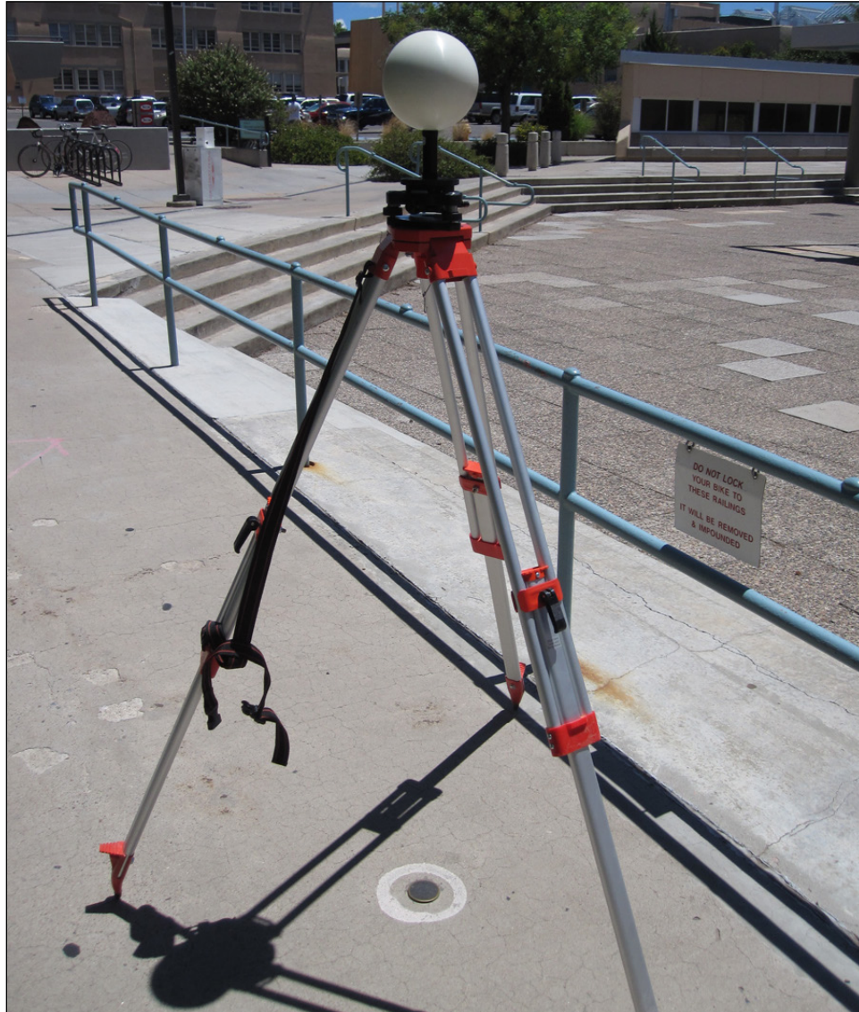
Figure 2-6 Typical Shape Target in LIDAR Surveys for MCLM or TLM
