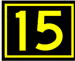
Figure 8. b. Runway Location Sign
