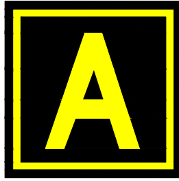
Figure 8. a. Taxiway Location Sign
