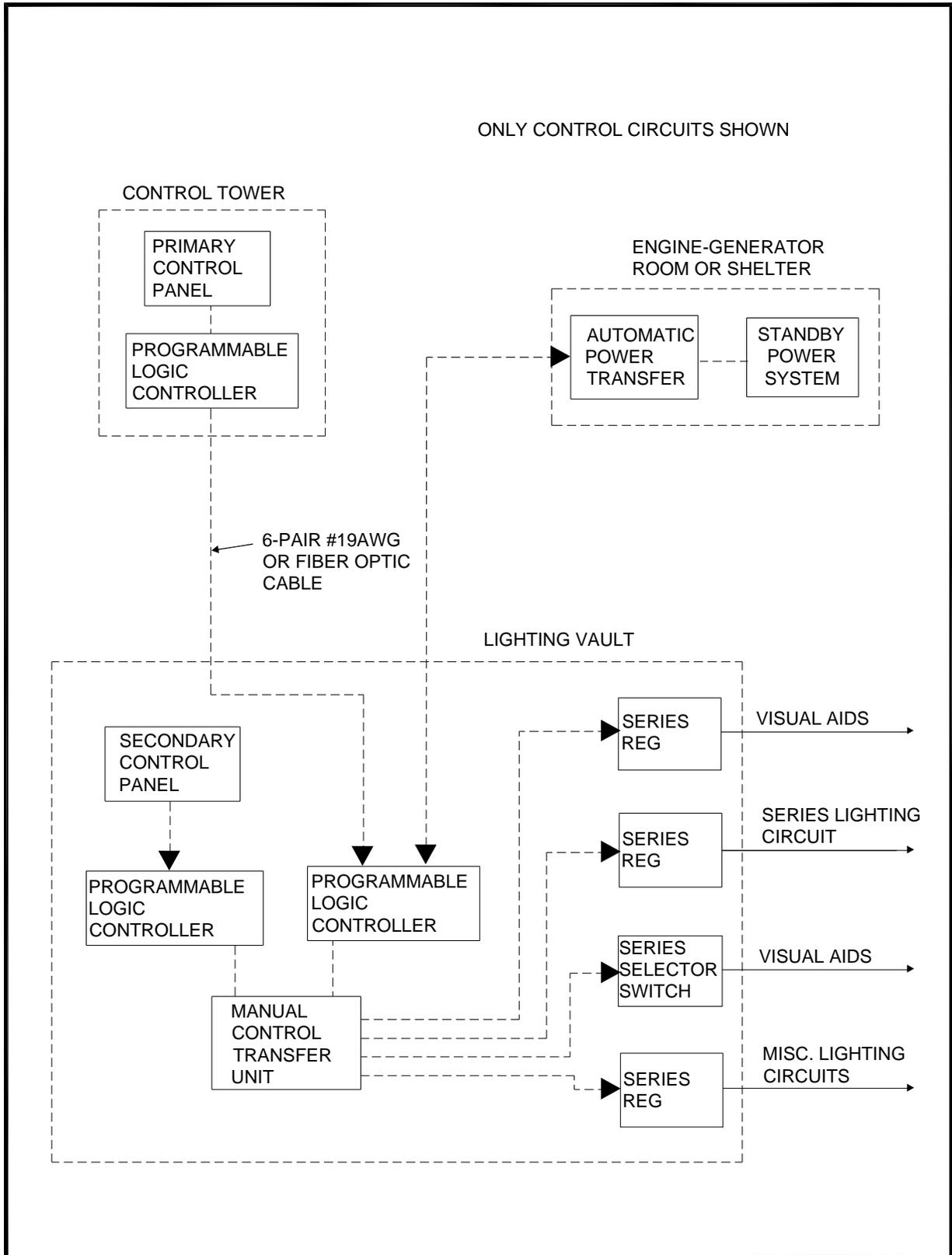
Figure 112. Typical PLC Control System Block Diagram
