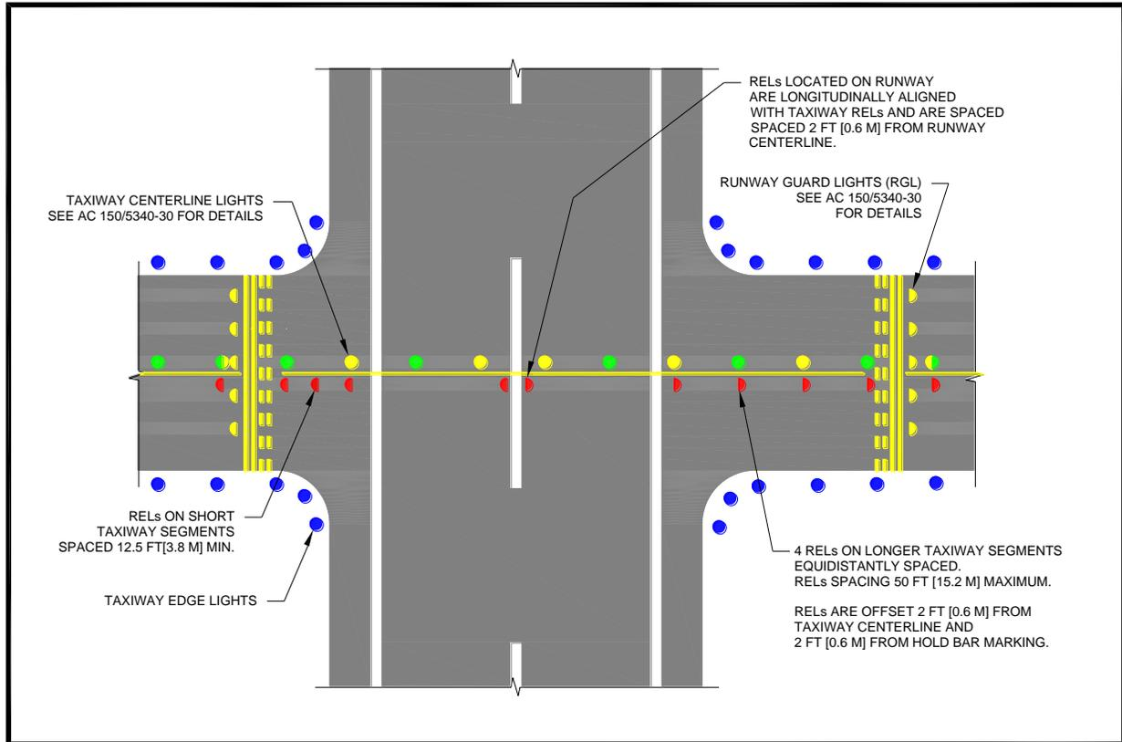
**Figure 144. REL Configuration for Taxiways at 90 Degrees**
