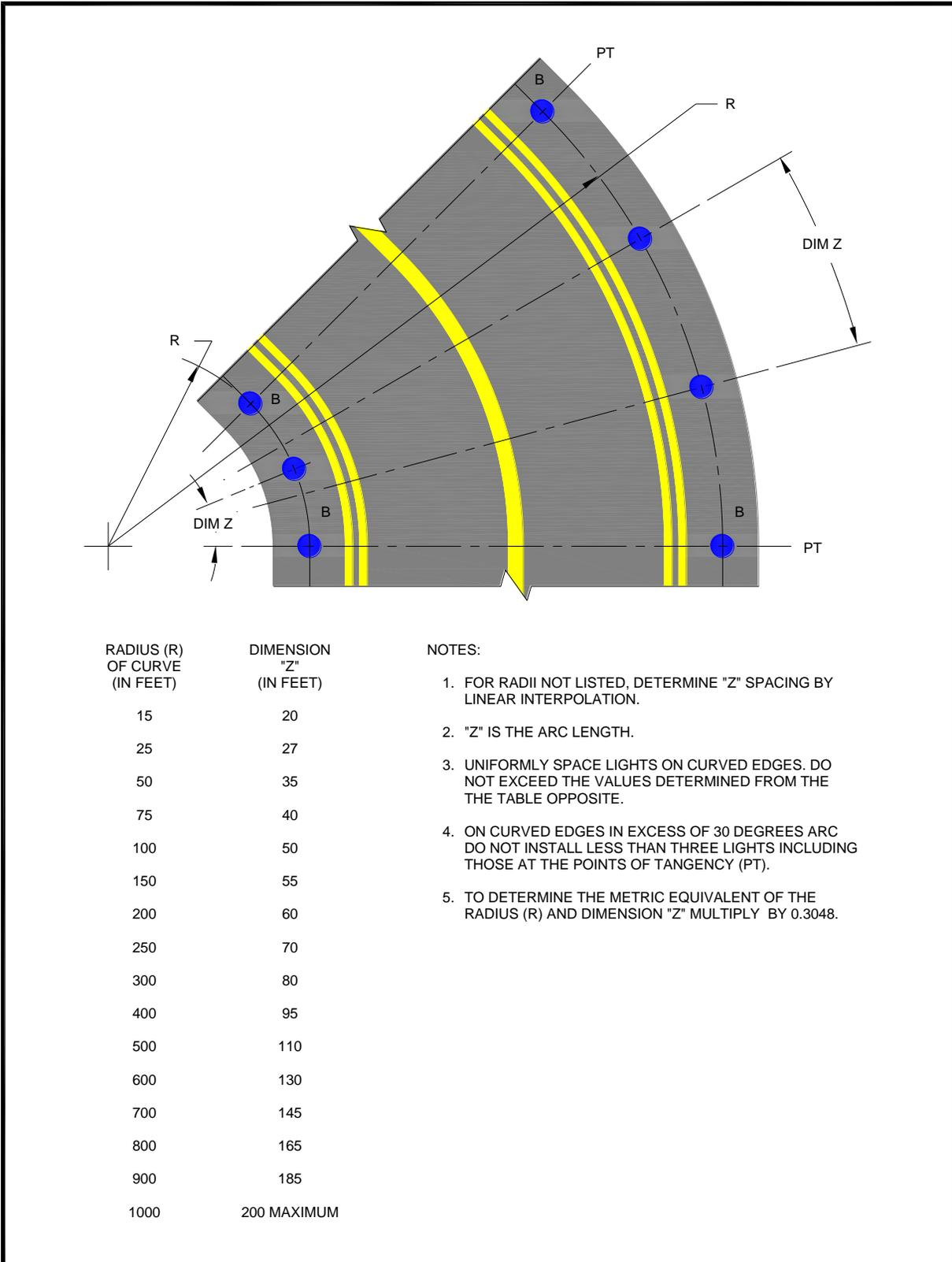
**Figure 17. Spacing of Lights on Curved Taxiway Edges**
