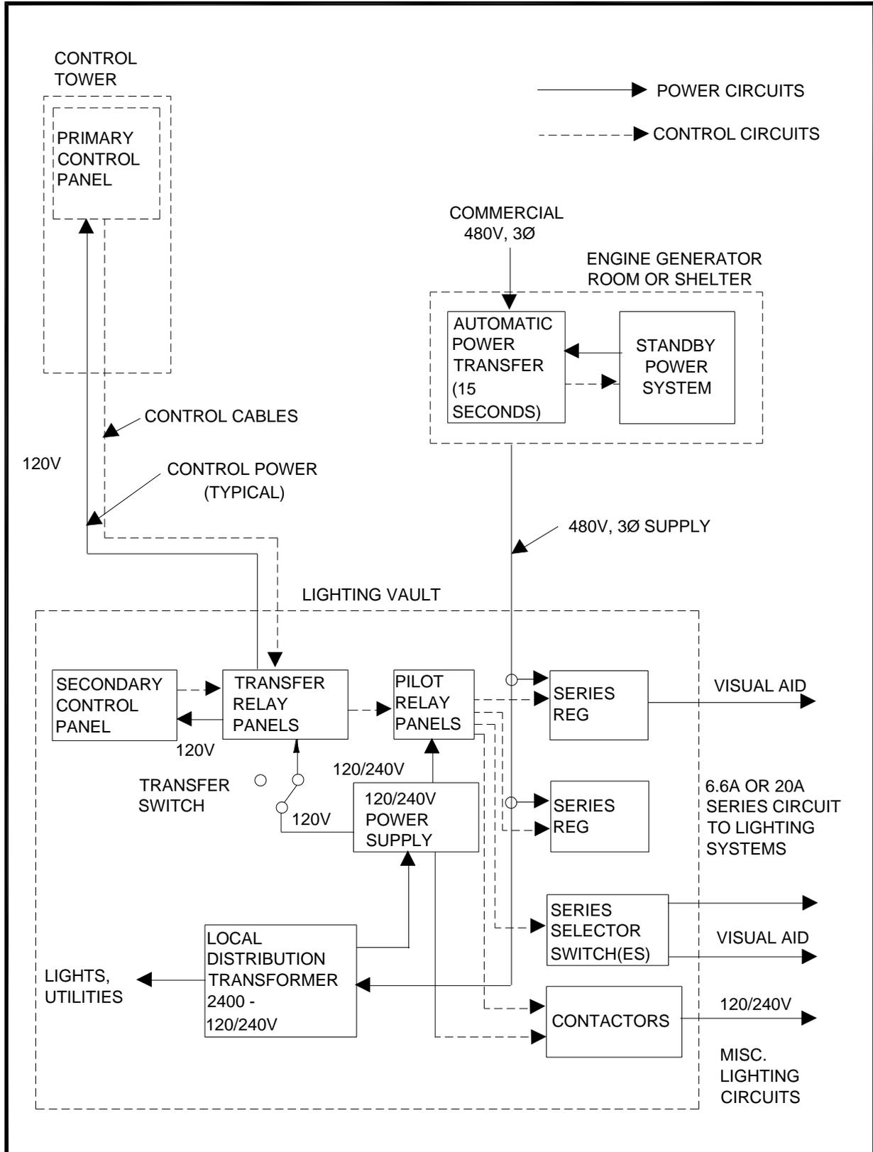
Figure 111. Power and Control System Block Diagram
