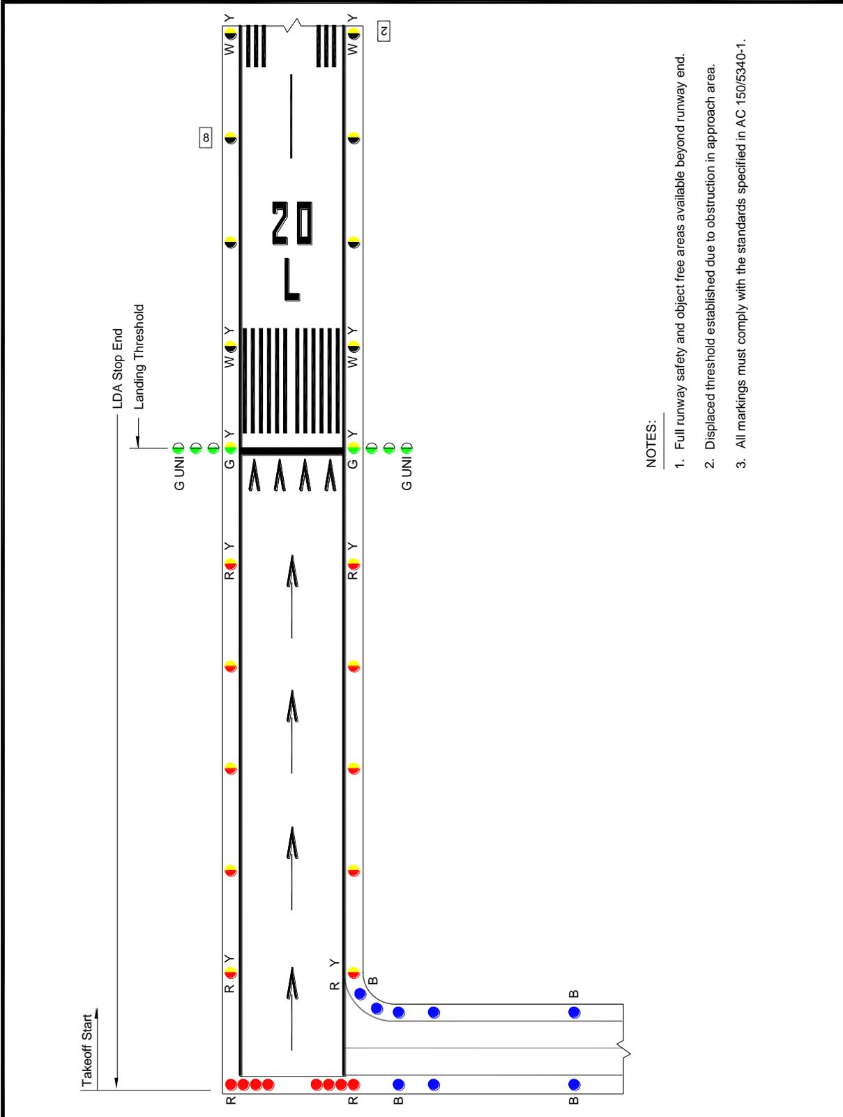
**Figure 6. Lighting for Runway with Displaced Threshold**
