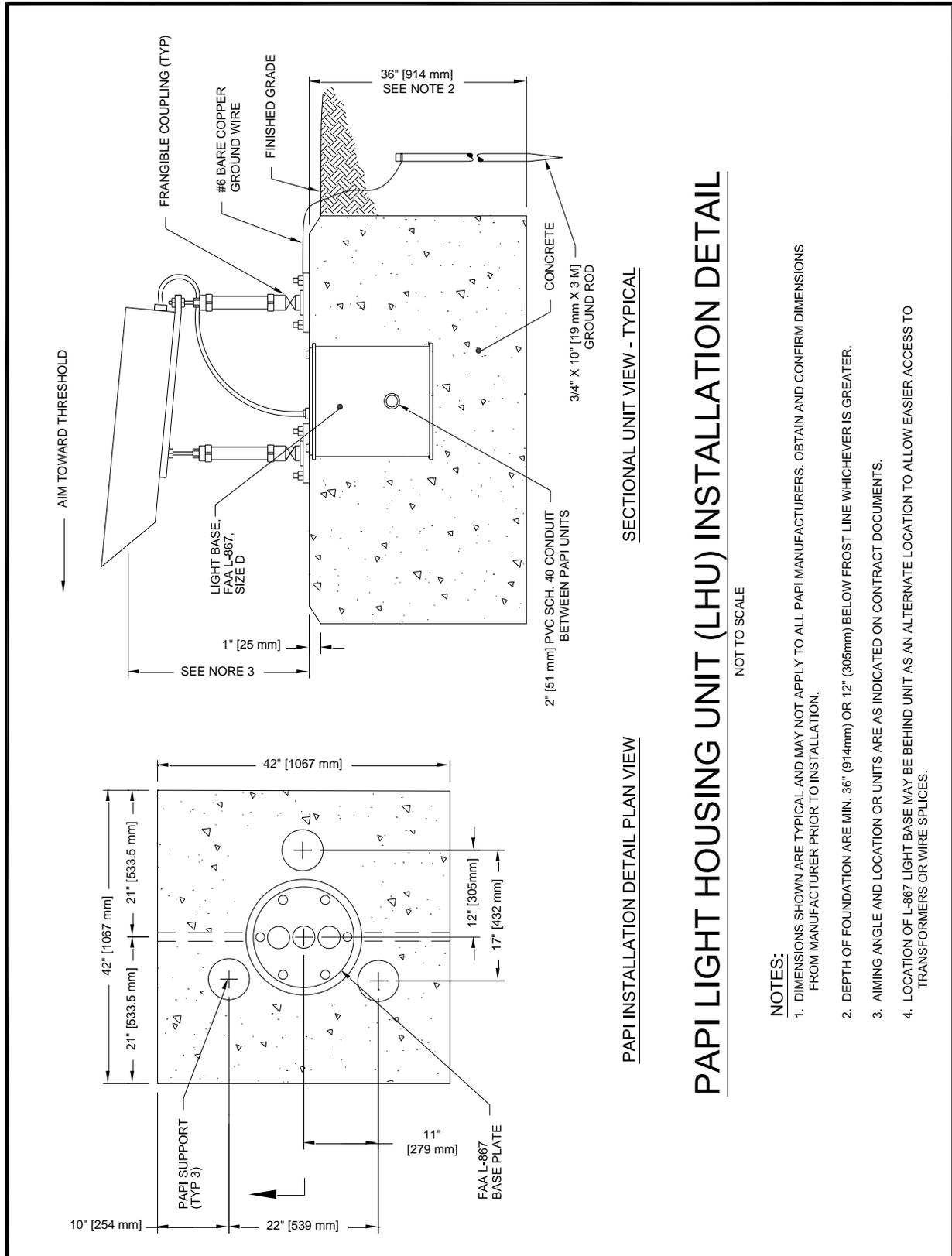
Figure 91. PAPI Light Housing Unit (LHU) Installation Detail
