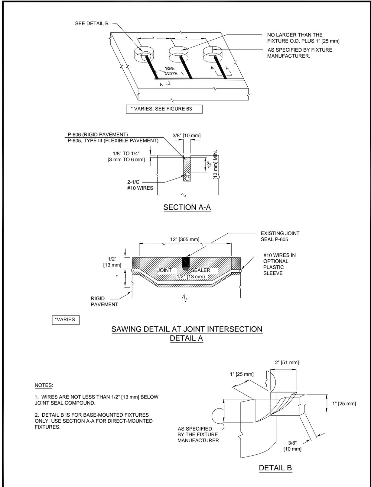
Figure 64. Sawing and Drilling Details for In-pavement Land and Hold Short Lights
