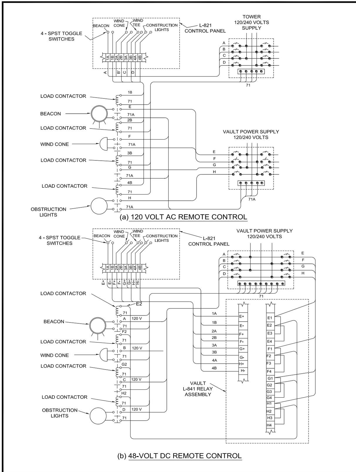
Figure 70. 120 Volt AC and 48 Volt DC Remote Control.
