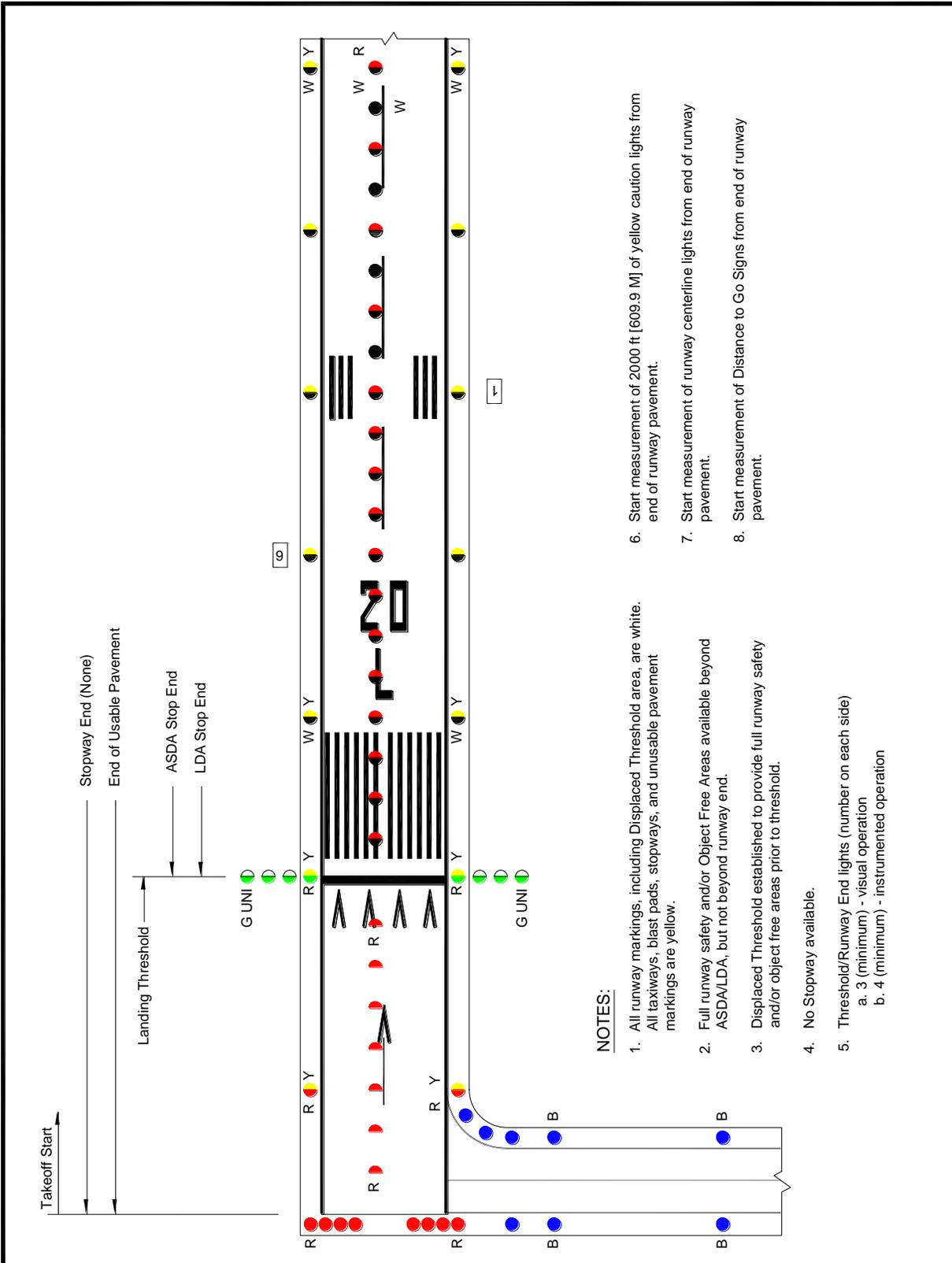
Figure 9. Lighting for Runway with Displaced Threshold/Usable Pavement
