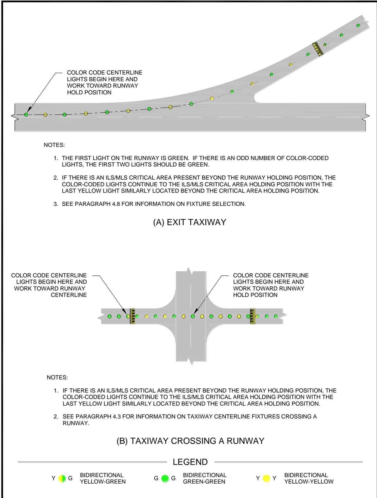
Figure 44. Color-Coding of Exit Taxiway Centerline Lights
