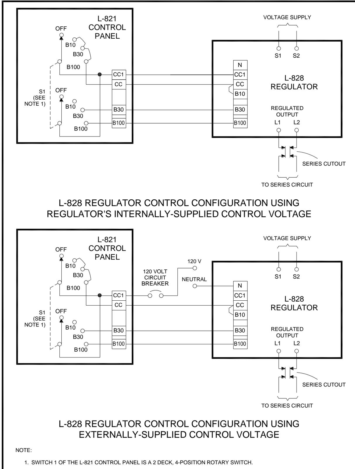
**Figure 27. Alternative 120 Volt AC Remote Control System**
