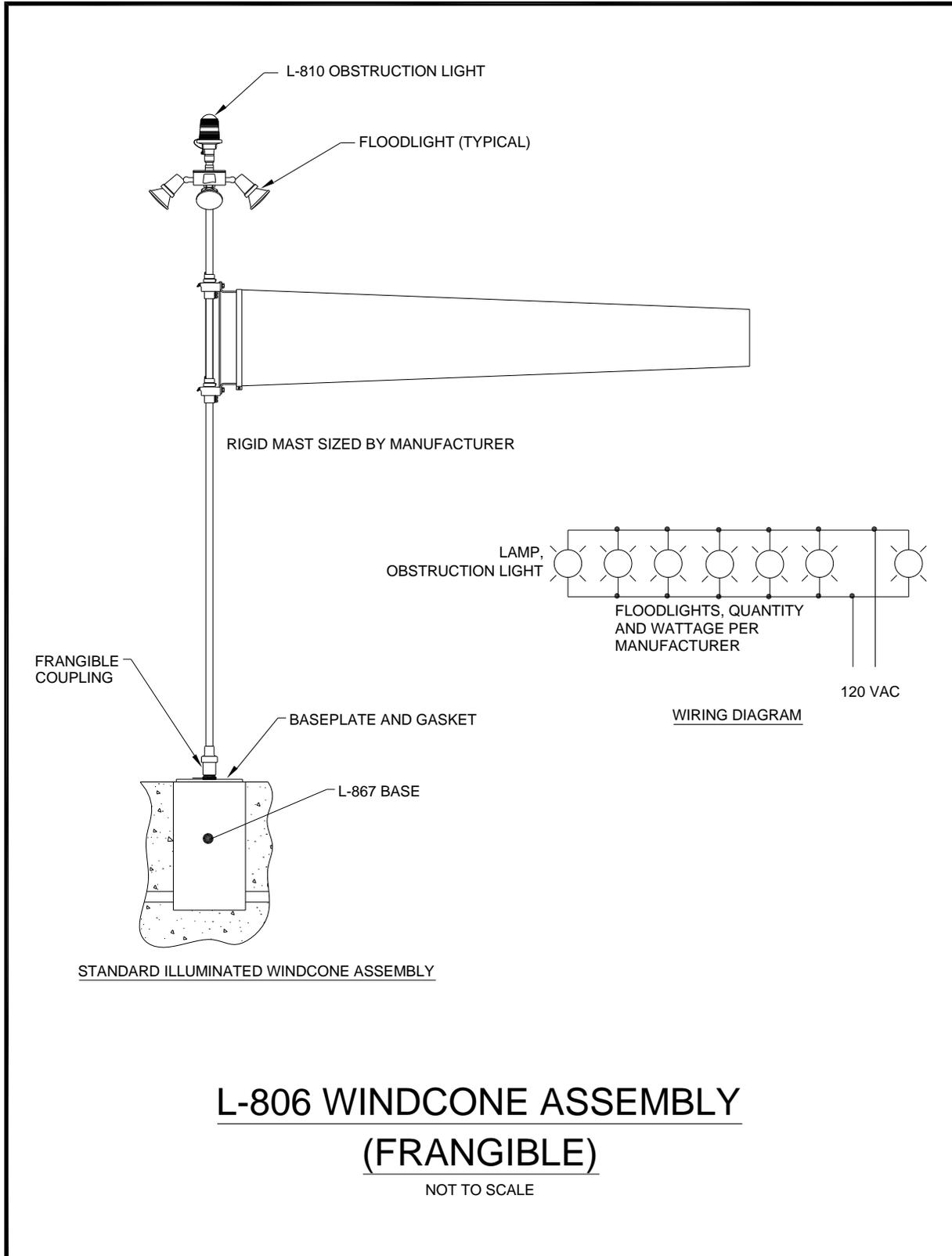
**Figure 76. Externally Lighted Wind Cone Assembly (Frangible)**
