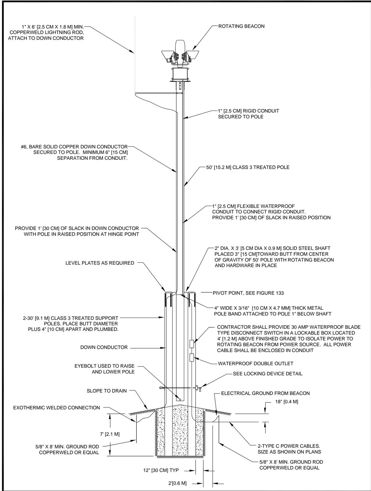
**Figure 131. Standard Details for Pivoting Rotating Beacon Pole**
