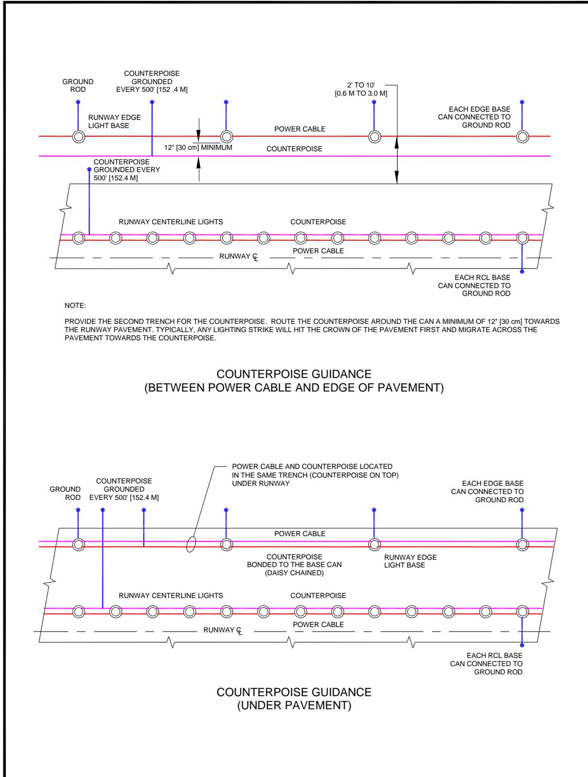
**Figure 117. Typical Counterpoise and Ground Rod Connections**
