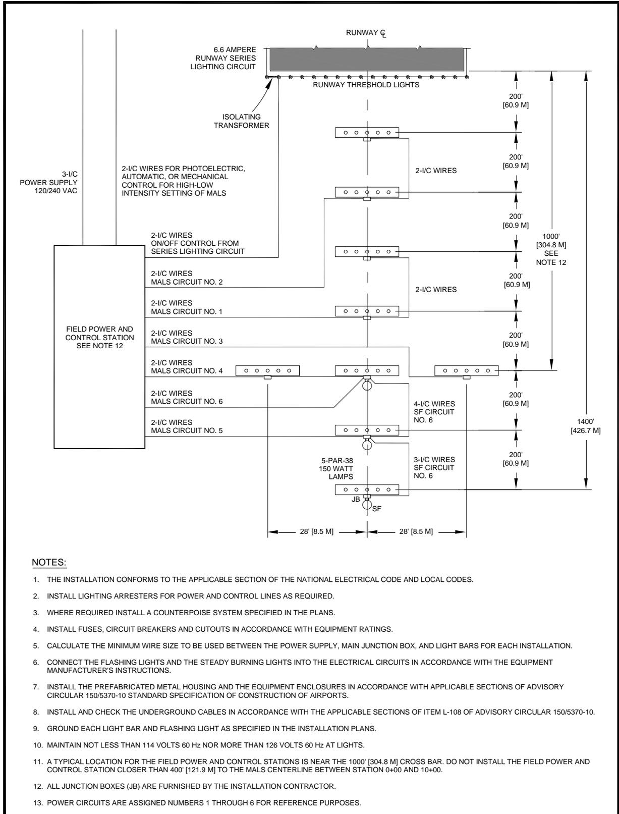
**Figure 85. Typical Field Wiring Circuits for MALSF**
