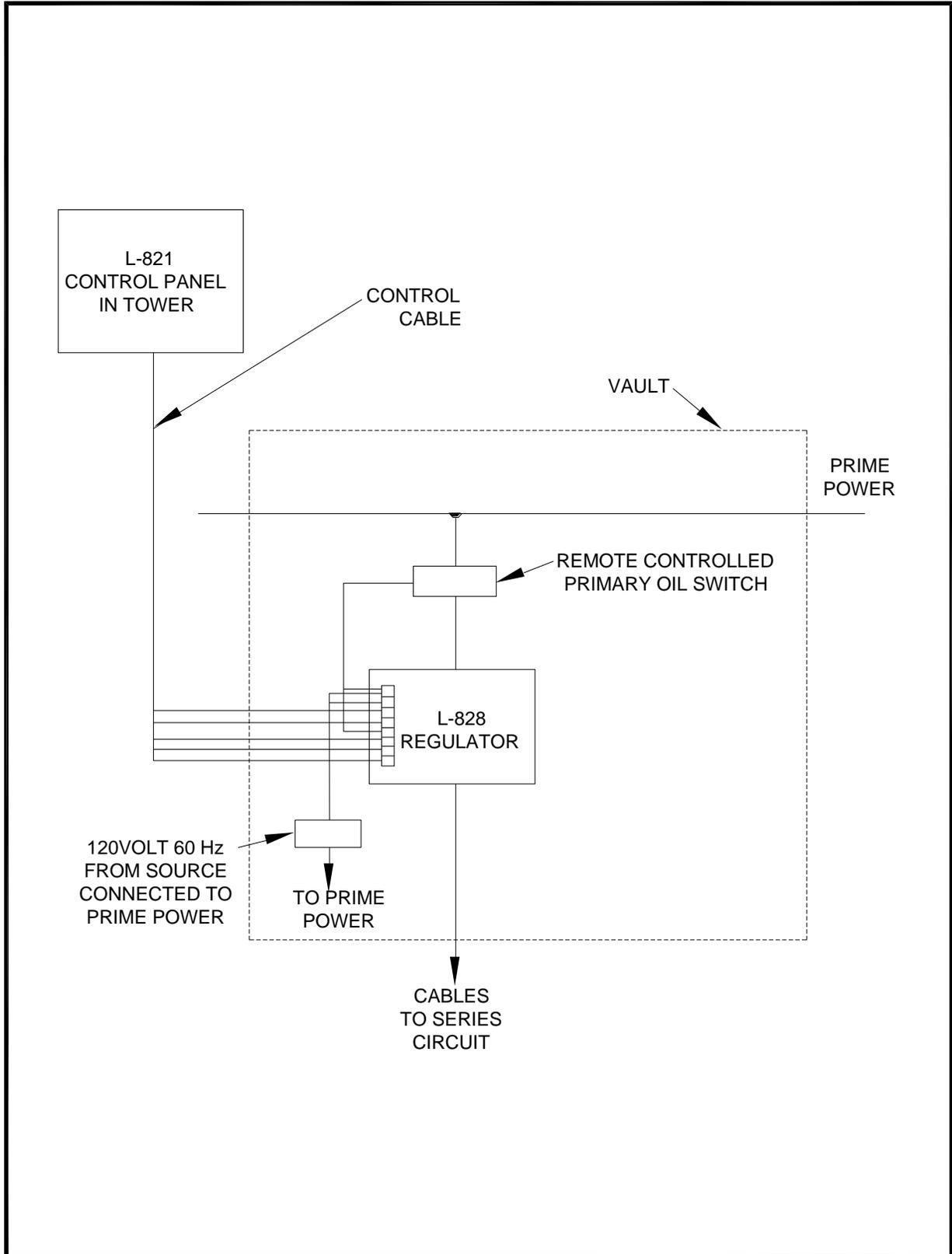
Figure 99. Typical Wiring Diagram for Configuration "C" Power
