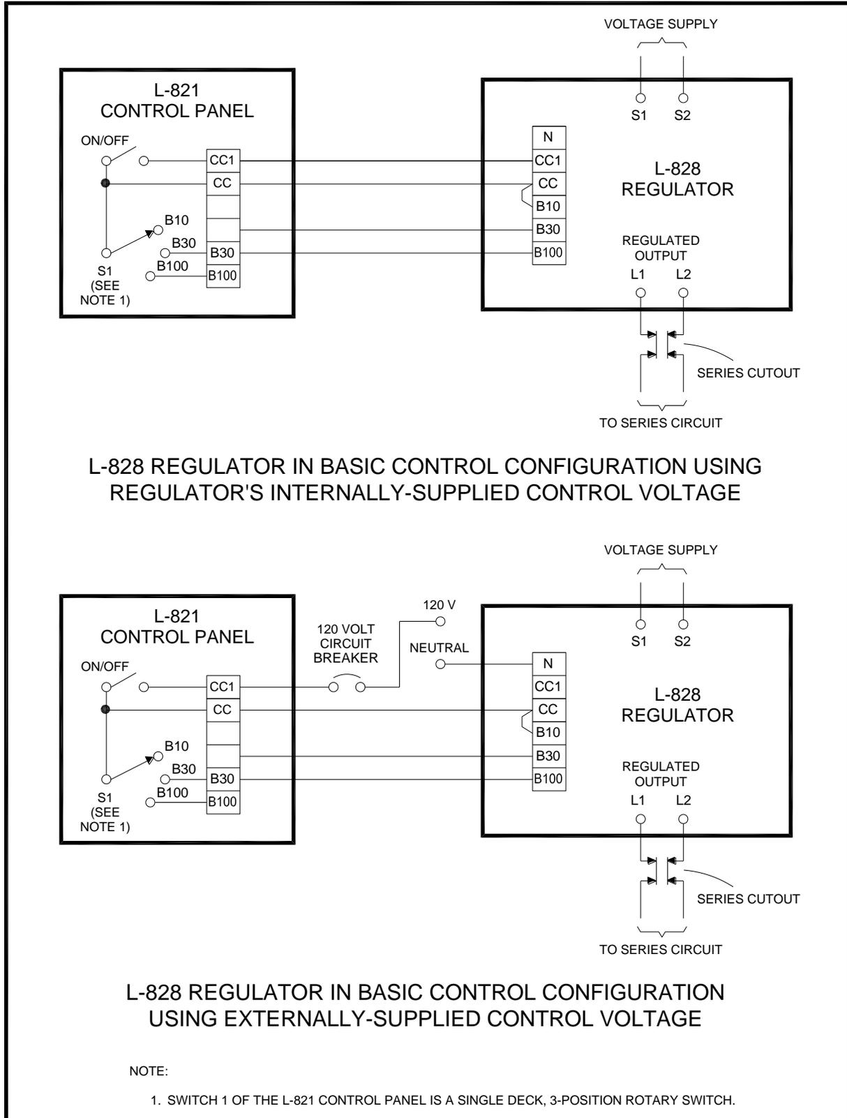
**Figure 26. Typical Basic 120 Volt AC Remote Control System**
