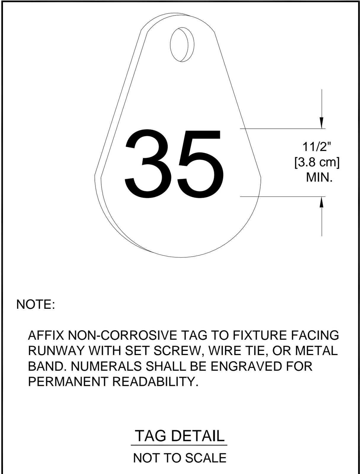
**Figure 118. Identification (ID) Tag Detail**
