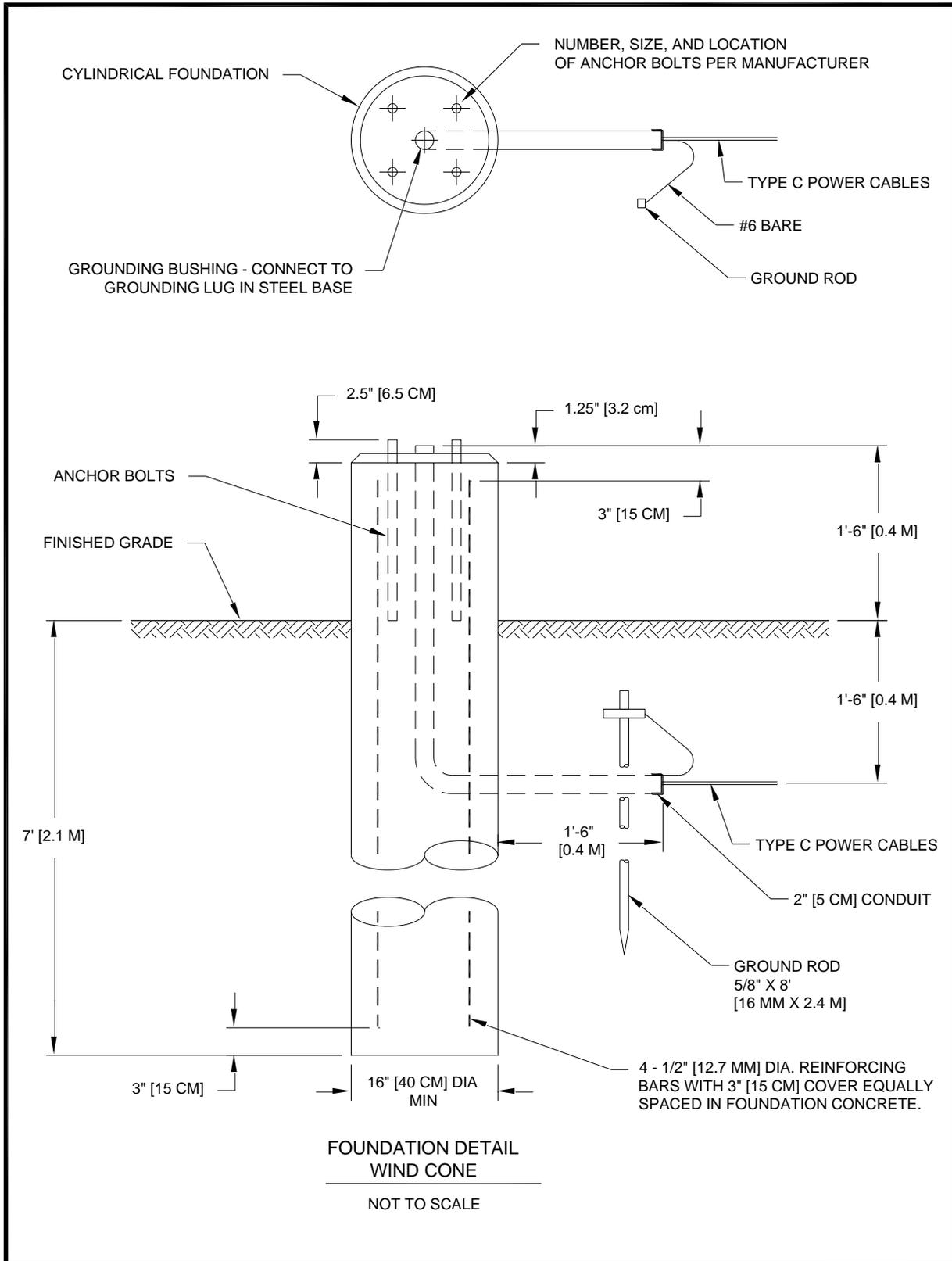
**Figure 132. Standard Details for Wind Cone Foundation (L-807)**
