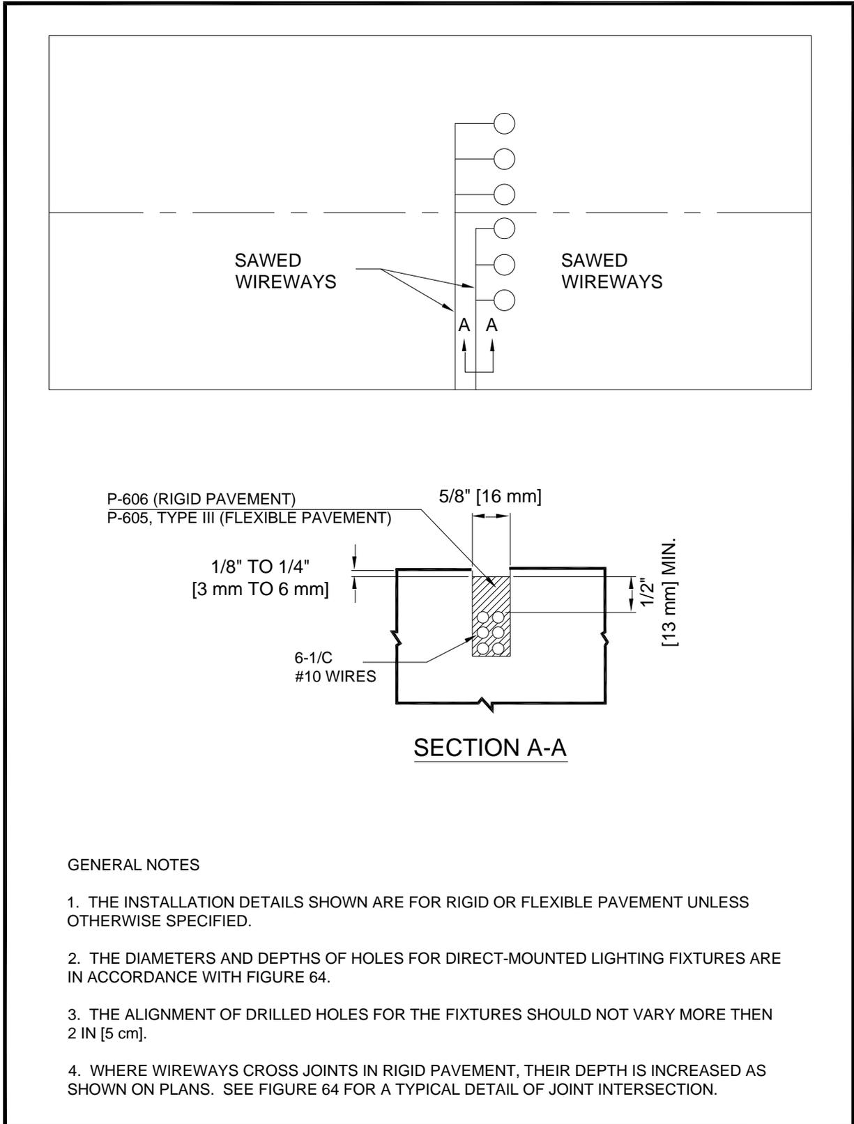
**Figure 63. Typical Wireway Installation Details for Land and Hold Short Lights**
