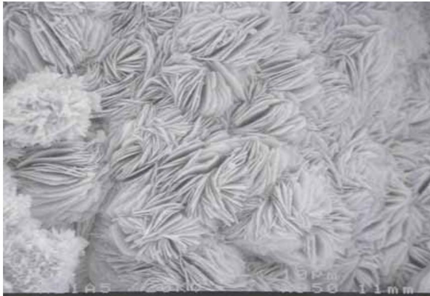
Figure 3-10. SEM image of rosette like crystalline ASR gel product.
