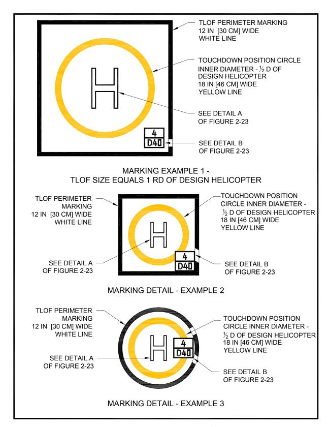
Figure 2–22. Standard and Alternate TLOF Marking: General Aviation
