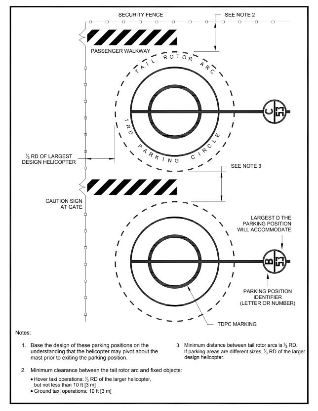
Figure 4-18. "Turn-around" Helicopter Parking Position Marking: Hospital
