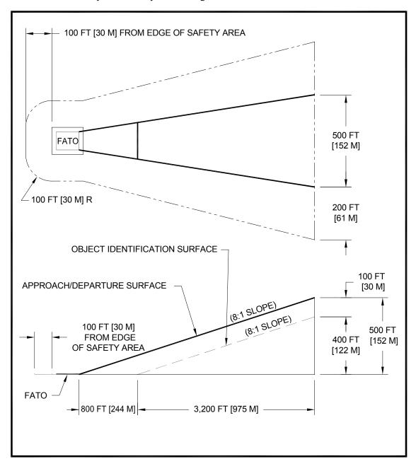
Figure 3–25. Airspace Where Marking and Lighting are Recommended:
