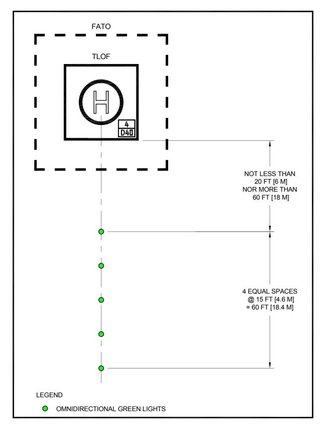
Figure 2-31. Landing Direction Lights: General Aviation
