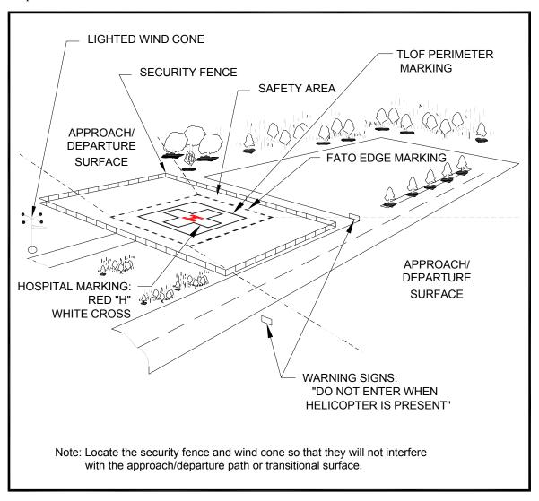
Figure 4-1. Essential Features of a Ground-level Hospital Heliport: Hospital
