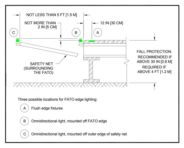
Figure 3-23. Elevated FATO - Perimeter Lighting: Transport
