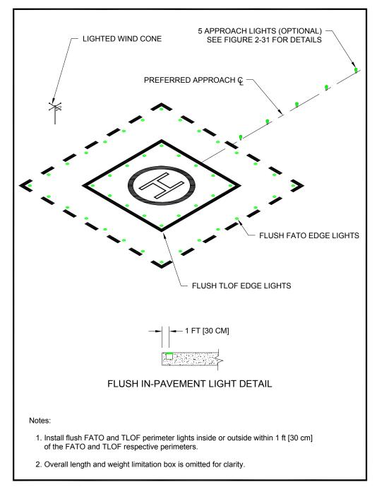
Figure 2-29. TLOF/FATO Flush Perimeter Lighting: General Aviation
