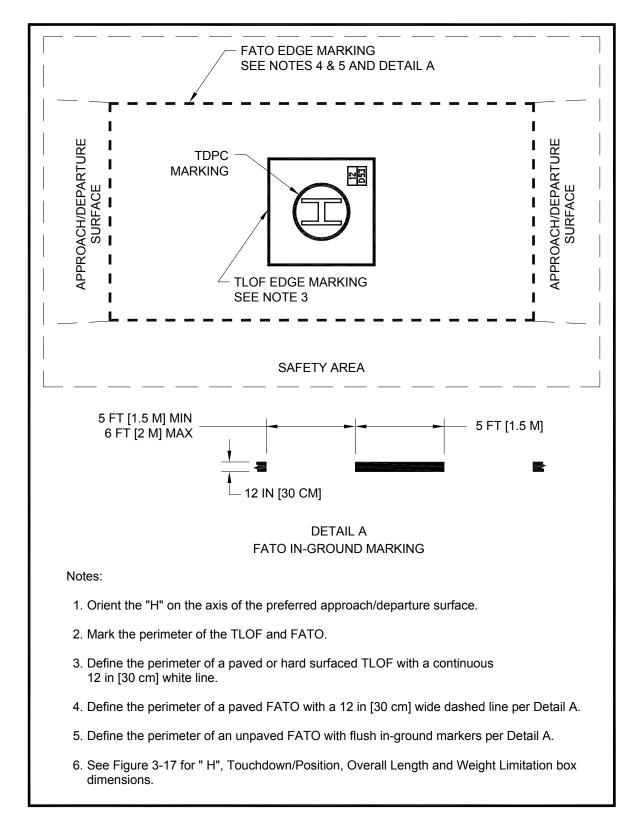
Figure 3–18. Paved TLOF/Paved FATO – Paved TLOF/Unpaved FATO – Marking: Transport
