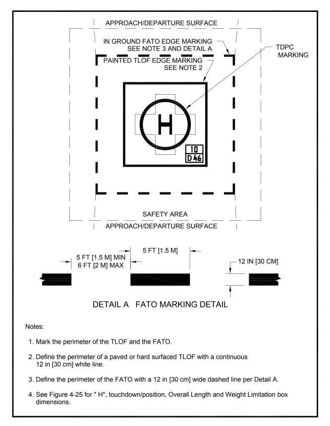
Figure 4-23. Paved TLOF/Paved FATO - Paved TLOF/Unpaved FATO - Marking: Hospital
