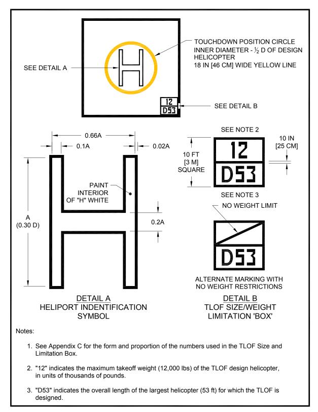
Figure 3–17. Standard Heliport Identification Symbol, TLOF Size and Weight Limitations: Transport
