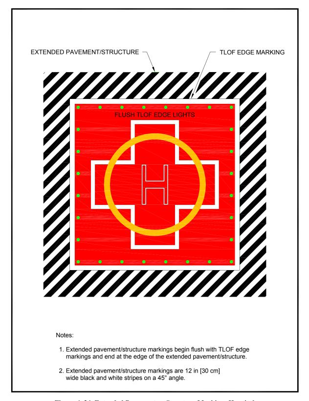
Figure 4-26. Extended Pavement or Structure Marking: Hospital
