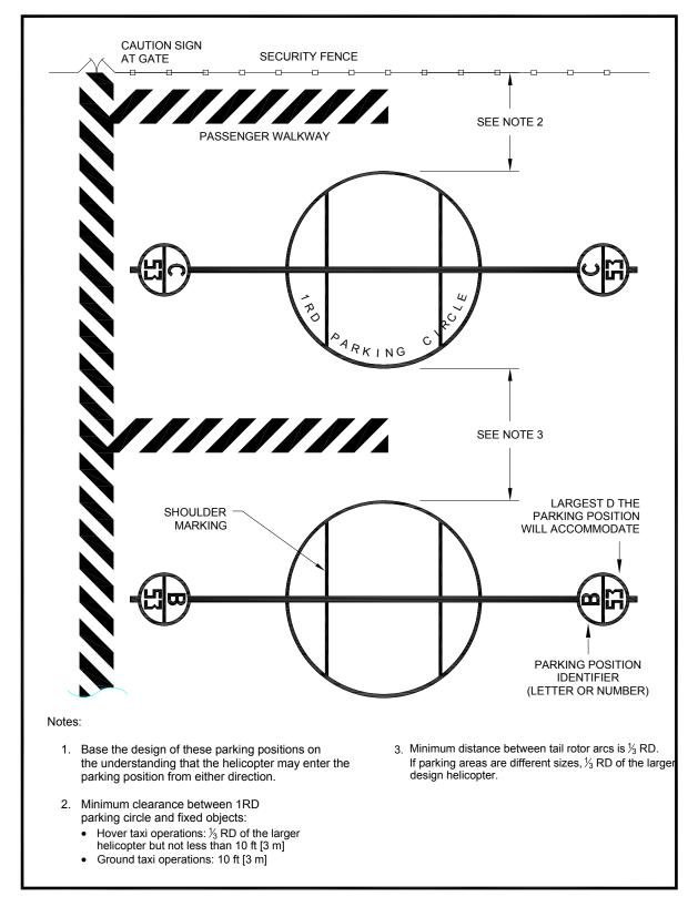
Figure 3-13. "Taxi-through" Helicopter Parking Position Marking: Transport
