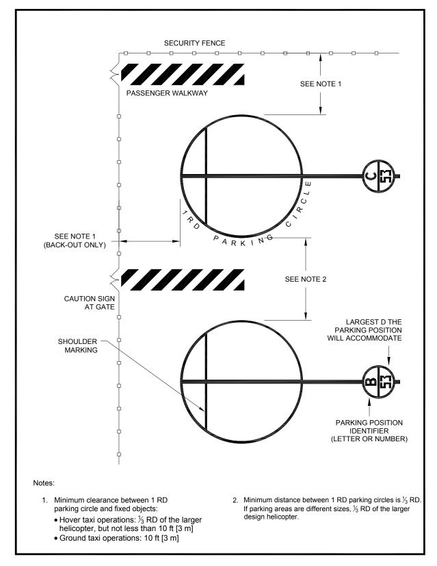
Figure 4-19. "Taxi-through" and "Back-out" Helicopter Parking Position Marking: Hospital
