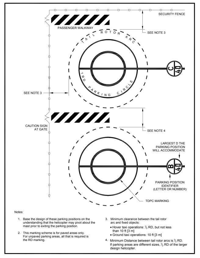
Figure 2-19. "Turn-around" Parking Position Marking: General Aviation
