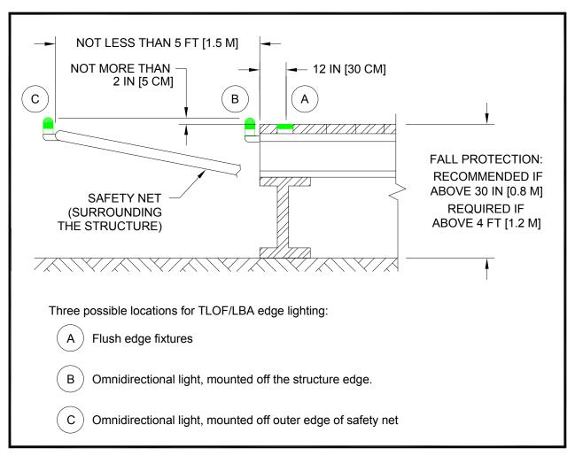
Figure 2-28. Elevated TLOF - Perimeter Lighting: General Aviation
