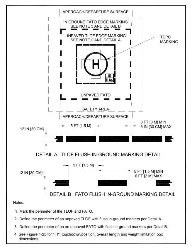
Figure 4-24. Unpaved TLOF/Unpaved FATO - Marking: Hospital
