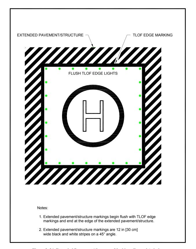
Figure 2-24. Extended Pavement / Structure Marking: General Aviation
