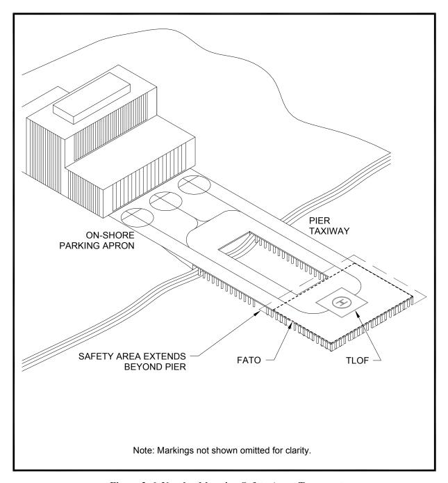
Figure 3-6. Non-load-bearing Safety Area: Transport
