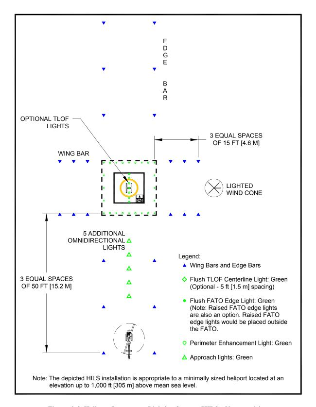
Figure 6-2. Heliport Instrument Lighting System (HILS): Non-precision
