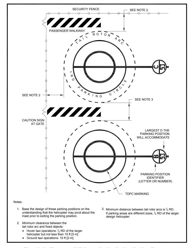
Figure 3–12. "Turn-around" Helicopter Parking Position Marking: Transport
