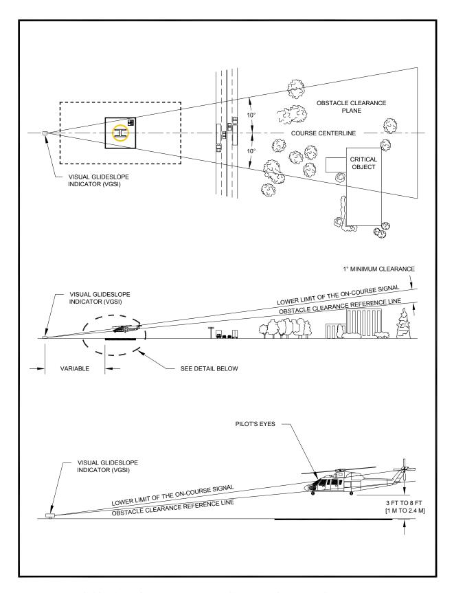
Figure 3-28. Visual Glideslope Indicator Siting and Clearance Criteria: Transport
