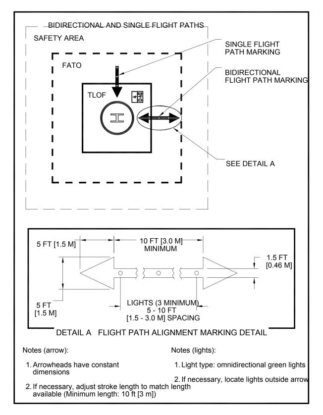
Figure 2-11. Flight Path Alignment Marking and Lights: General Aviation
