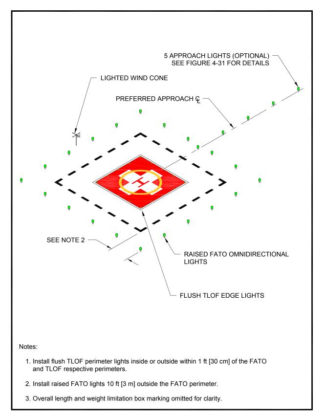
Figure 4-30. Flush TLOF and Raised FATO Perimeter Lighting: Hospital
