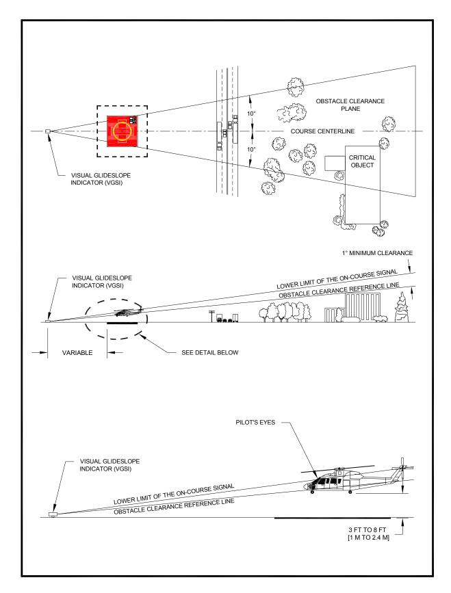
Figure 4-35. Visual Glideslope Indicator Siting and Clearance Criteria: Hospital
