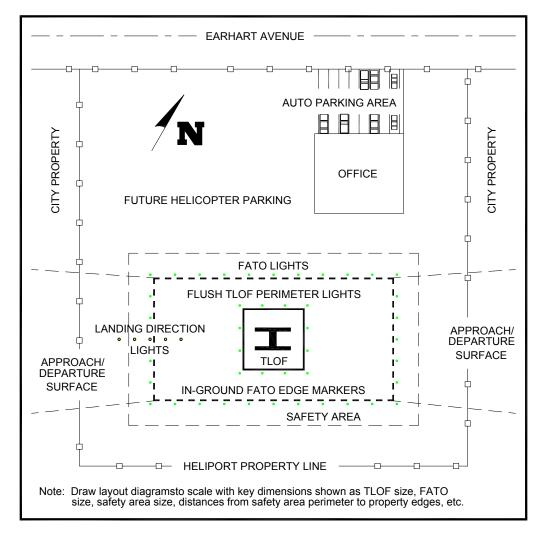
Figure 1-2. Example of a Heliport Layout Plan
