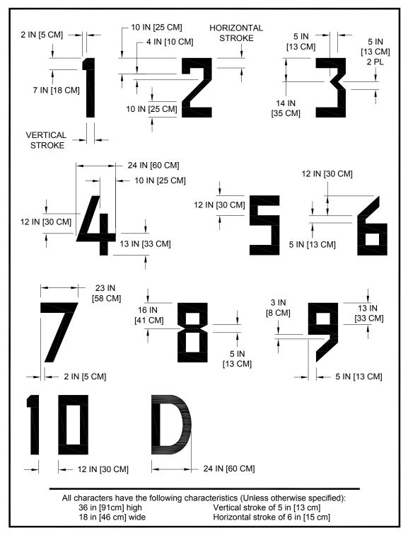
Figure C-1. Form and Proportions of 36 Inch (91 cm) Numbers for Marking Size and Weight Limitations
