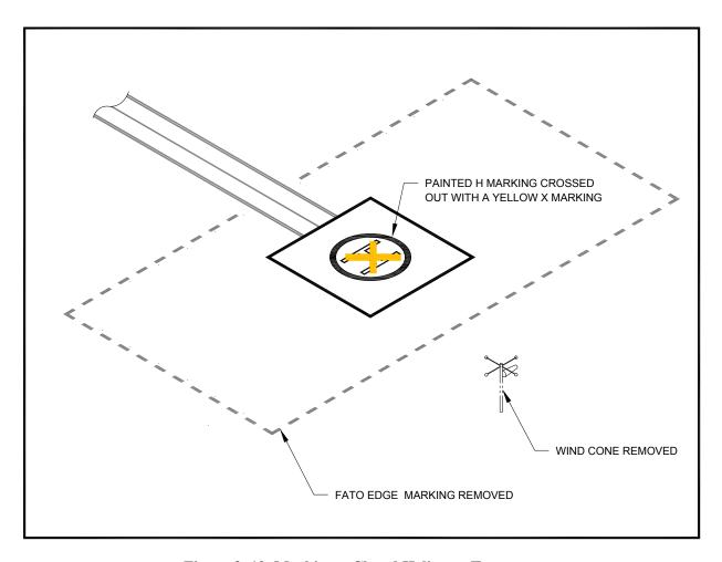
Figure 3-19. Marking a Closed Heliport: Transport
