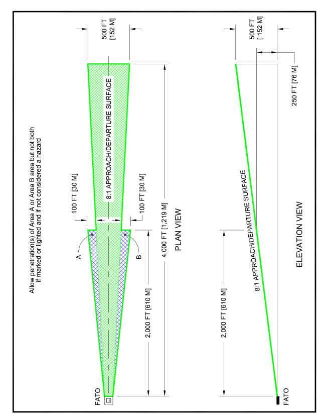
Figure 2–9. VFR PPR Heliport Lateral Extension of the 8:1 Approach / Departure Surface: General Aviation
