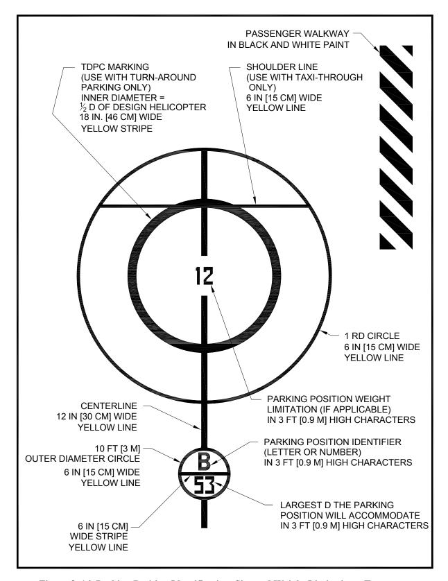
Figure 3-16. Parking Position Identification, Size and Weight Limitations: Transport
