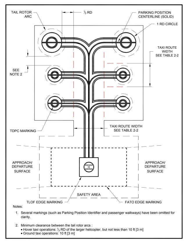
Figure 3-14. Parking Area Design - "Turn-around" Parking Positions: Transport
