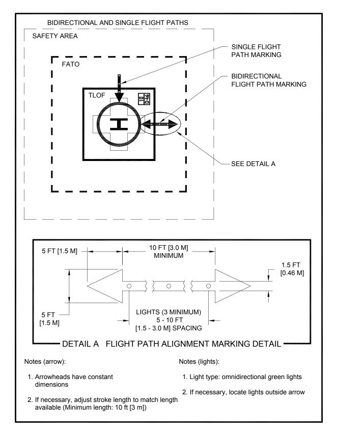
Figure 4-10. Flight Path Alignment Marking and Lights: Hospital
