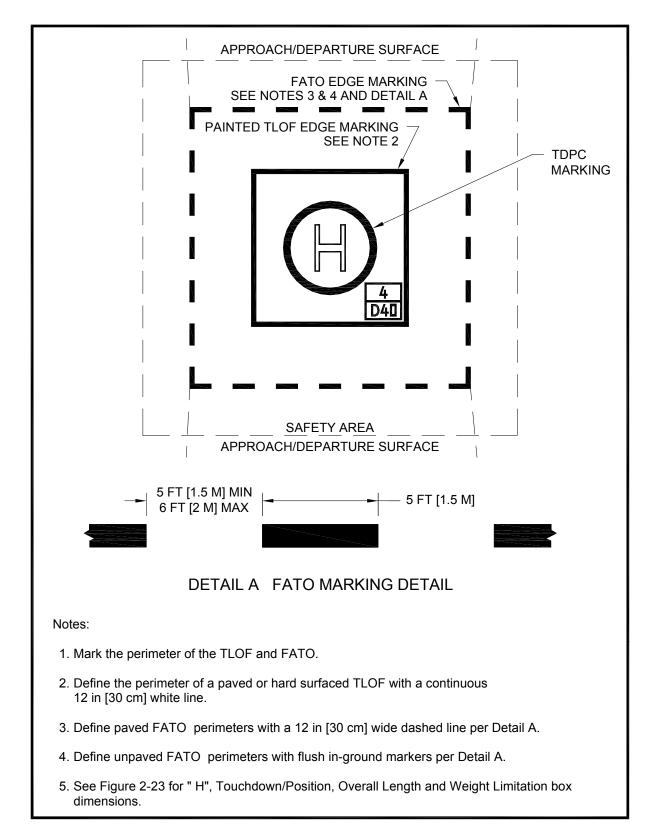
Figure 2–25. Paved TLOF/Paved FATO – Paved TLOF/ Unpaved FATO – Marking: General Aviation
