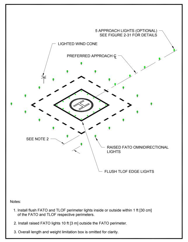
Figure 2-30. TLOF Flush and FATO Raised Perimeter Lighting: General Aviation
