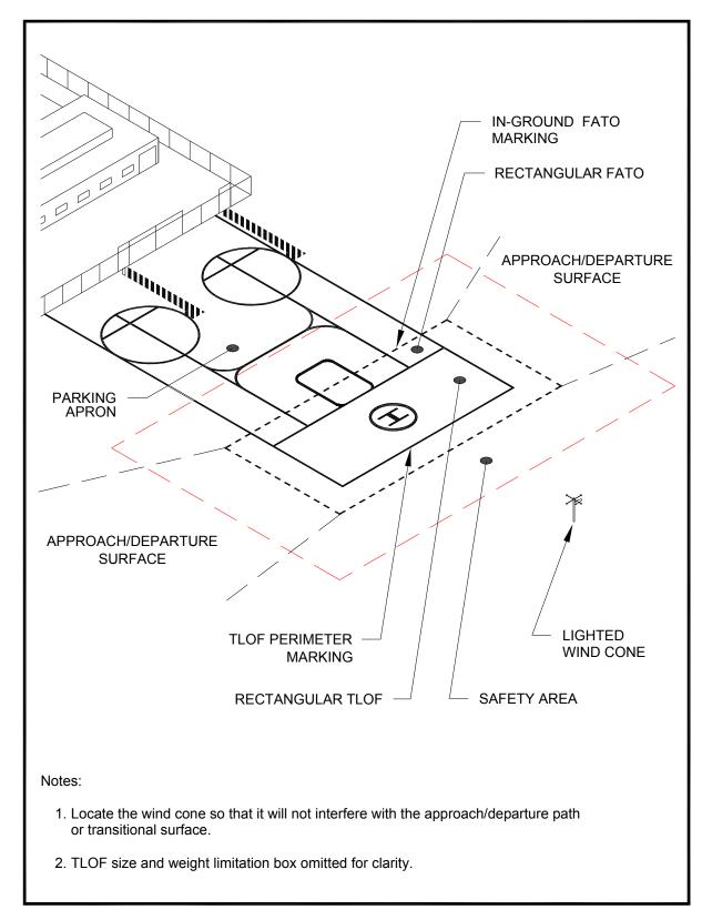
Figure 3–1. Typical Transport Heliport: Transport
