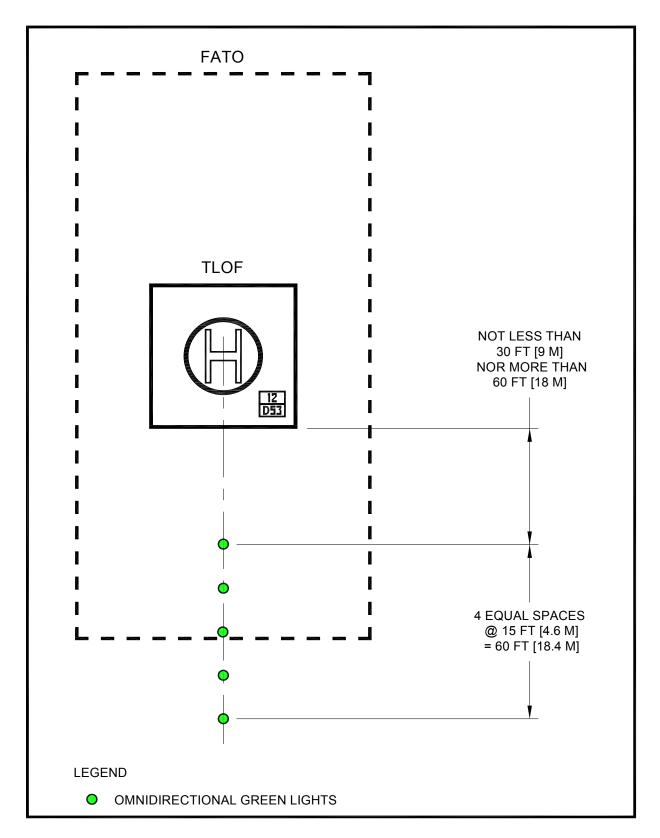
Figure 3–24. Landing Direction Lights: Transport
