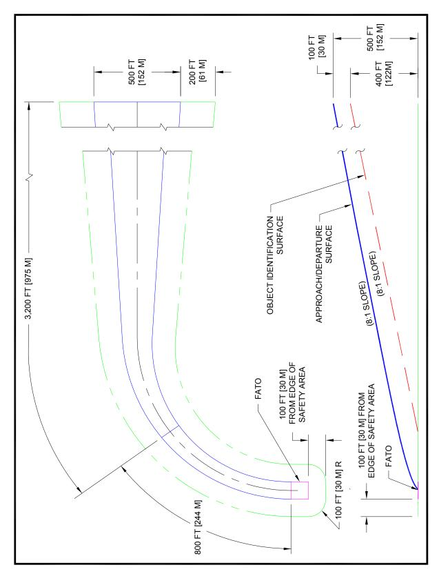
Figure 3–26. Airspace Where Marking and Lighting are Recommended: Curved Approach: Transport
