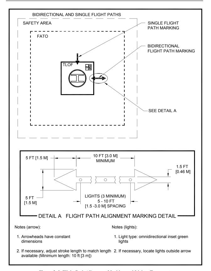
Figure 3-9. Flight Path Alignment Marking and Lights: Transport
