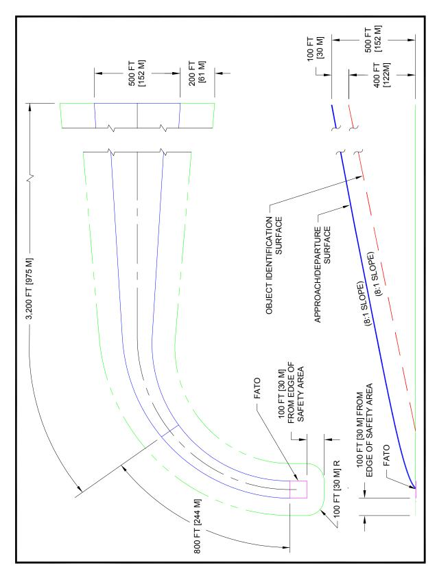
Figure 2–33. Airspace Where Marking and Lighting are Recommended: Curved Approach: General Aviation
