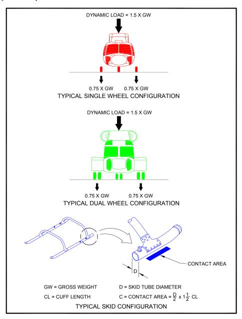
Figure 7-2. Helicopter Landing Gear Loading: Gradients and Pavement
