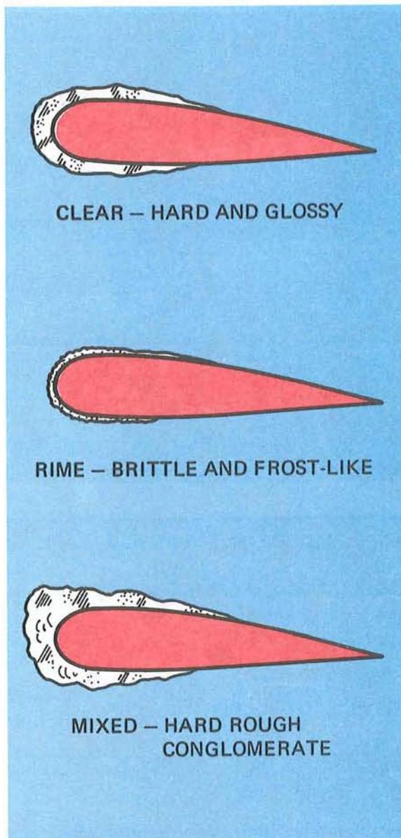
FIGURE 90. Clear, rime, and mixed icing on airfoils.
