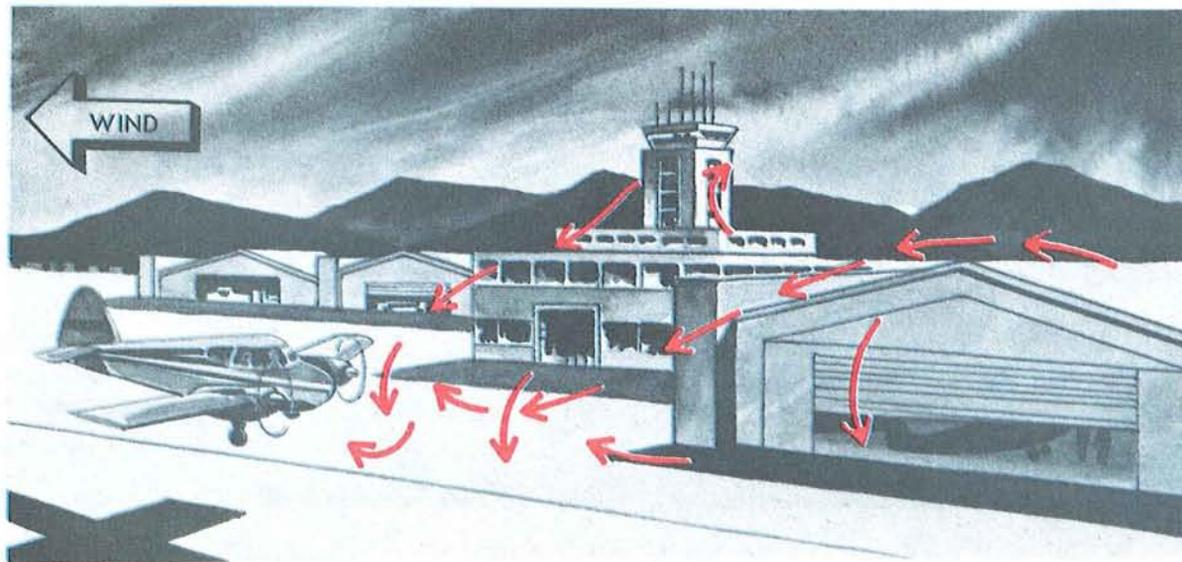
FIGURE 79. Turbulent air in the landing area.
