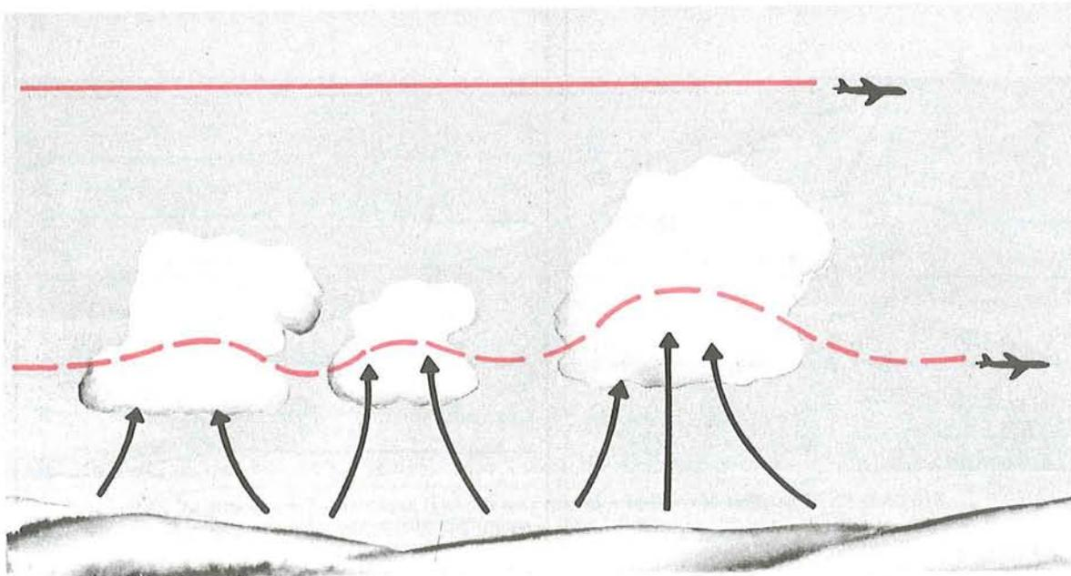
FIGURE 77. Avoiding turbulence by flying above convective clouds.
