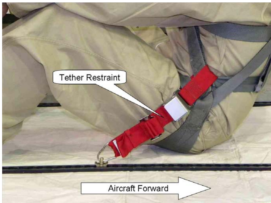
FIGURE 6. TETHER RESTRAINT ATTACHMENT TO FLOOR FOR REAR-FACING FLOOR SEATS
