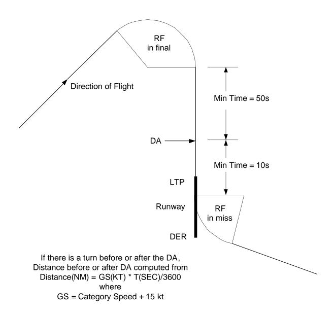
Figure 1. Minimum Straight Path Before DA
