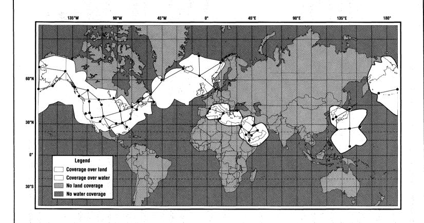
Contours represent the range limits in which the signal-to-noise ratio (SNR) falls to 1:3 (or -10 db SNR) and the accuracy limits in which the GDOP falls to 7,700 ft/ $\mu s$ .
