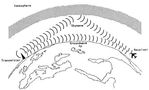
The Loran-C sky wave signal (—) is reflected earthward from the ionosphere, requiring a longer time to reach the aircraft than the ground wave (- - -).
