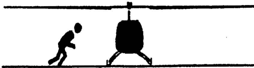
FIGURE 4. CROUCH UNDER THE MAIN ROTOR
