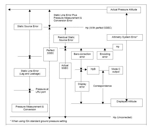
FIGURE 2-1. ALTIMETRY SYSTEM ERROR AND ITS COMPONENTS
