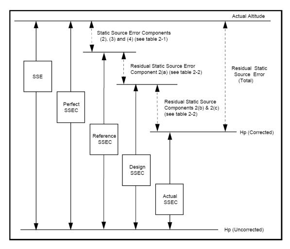
(d) Account for factors that create variability of SSE relative to the reference characteristic in two ways. First, as noted for the SSE itself in Table 2-1, and second, for its effect on the application of SSEC as in factor 2(a)(i) of Table 2-2. Similarly, account for the static pressure measurement error in two separate ways. The main effect will be via the "pressure measurement and conversion" component, but a secondary effect will be via factor 2(a)(ii) Table 2-2.
