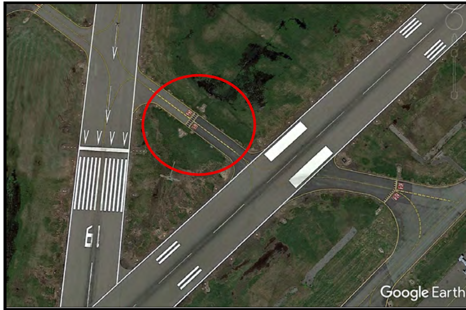
Figure J-31. Taxiway Connections to V-shaped Runways
