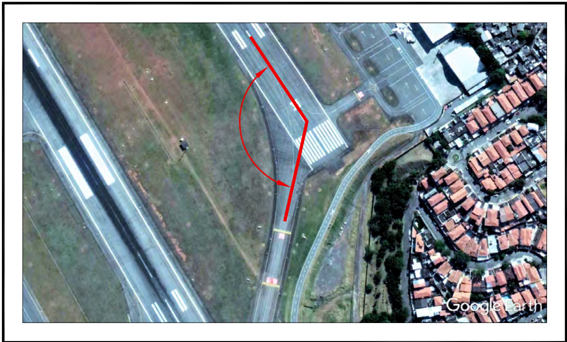
Figure J-15. Entrance Taxiway Intersecting Runway End at an Angle Greater Than 90 Degrees
