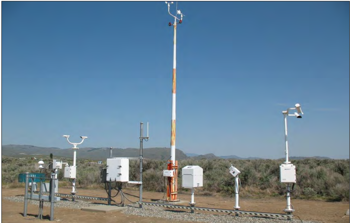
Figure 6-25. Automated Surface Observing System (ASOS) Weather Sensors Suite
