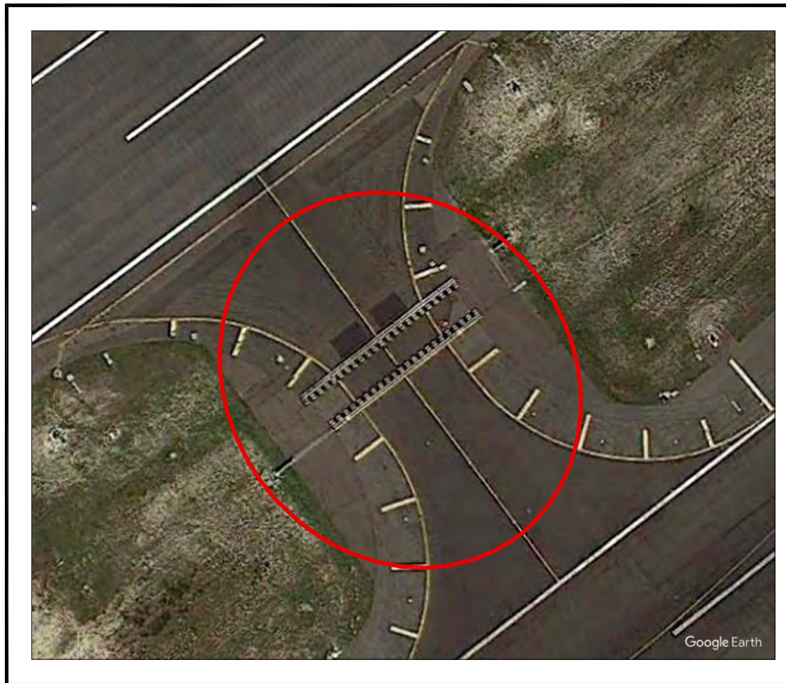
Figure J-25. Aerial Image of Short (Stub) Taxiway Connection to a Runway
