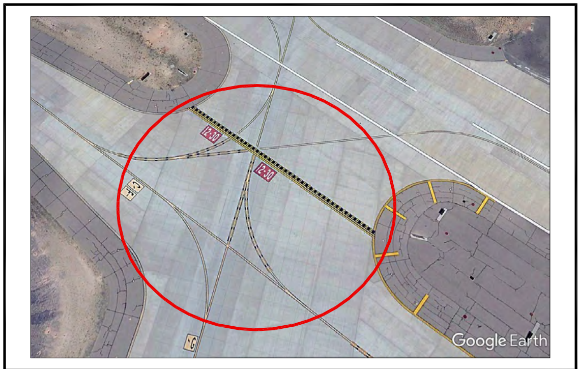
Figure J-16. Aerial Image of Complex Taxiway Intersection Exceeding the “Three-Path” Concept
